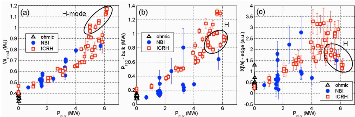
**FIGURE 2.** Comparison of NBI and N=2 ICRF heating performance in L-mode hydrogen plasmas in JET-ILW: (a) plasma stored energy (EFIT); (b) bulk plasma radiation (bolometer); (c) edge W concentration (VUV spectroscopy).
