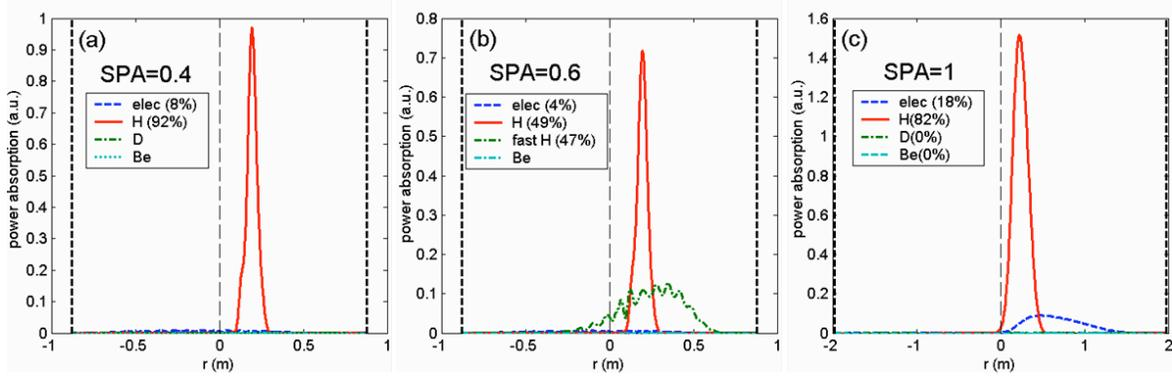
**FIGURE 1.** ICRF simulations of N=2 H majority ICRH ( $B_0=1.8\text{T}$ ,  $f=51.5\text{MHz}$ ): (a) JET experimental parameters; (b) JET parameters with 2% of fast H ions at 100keV; (c) ITER half-field parameters. Traces of D and Be were also considered in the simulations.
