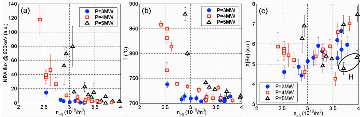
**FIGURE 4.** Fast ion acceleration and impact on plasma-wall interaction as function of the plasma density for various ICRF power levels: (a) NPA hydrogen flux at  $E_H=600\text{keV}$ ; (b) Poloidal limiter temperature (IR camera); (c) Edge Be concentration (visible spectroscopy).
