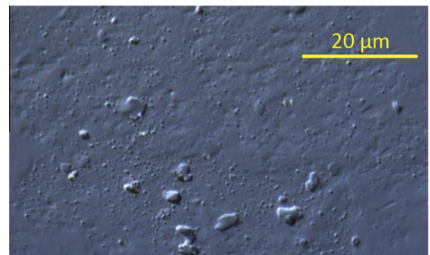
Fig. 2. Optical image of the surface of the pre-exposed W sample.
