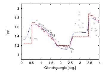
Fig. 6. Comparison of the experimental and theoretical phase of oscillations. Experimental data collected by Crook *et al.* (1989) are shown with crosses. Theoretical results obtained by the direct examination of oscillations runs are shown with the solid line, theoretical results obtained using harmonic analysis are shown with the dotted line. Thermal vibrations of atoms were ignored in the theoretical model.
