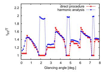
Fig. 5. Plots of the oscillation phase determined using two different methods (direct and employing the Fourier series, respectively) for the identical sets of theoretical oscillations,  $N_{cov} = 20$ .
