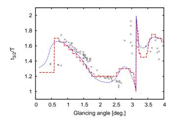
Fig. 7. The same as for Fig.6, however, theoretical results are for the model taking into account thermal vibrations of atoms. The following vaules of Debye-Waller factors were assumed:  $B_{Ga}=2.0~\text{Å}^2$  and  $B_{As}=2.7~\text{Å}^2$ .
