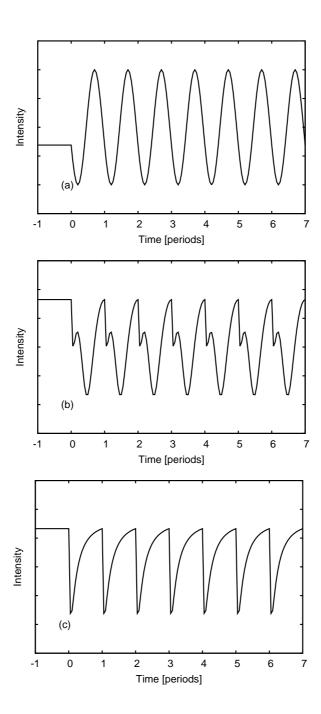
Fig. 2. Runs of oscillations which need to be admitted in theoretical work: (a) oscillations which can be described with the help a cosinus-like function, (b) oscillations with double minima and maxima in one period, (c) the intensity changes which are strongly asymmetric within one period.
