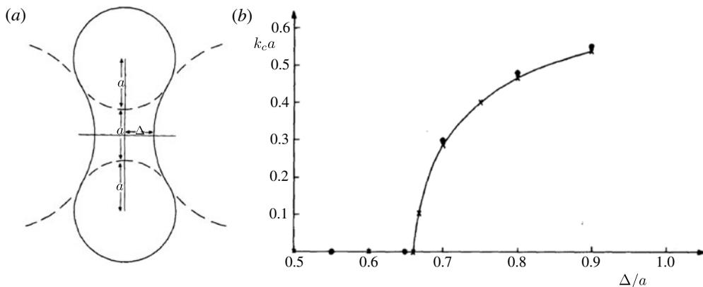
FIGURE 28. (a) Idealised multipinch and (b) toroidal wavenumber corresponding to the lowest eigenvalue as a function of  $\Delta$ . (Reproduced with permission from Gimblett *et al.* (1987). Copyright 1987, AIP Publishing LLC.)
