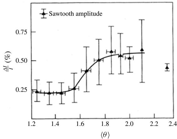
FIGURE 25. Driving a toroidal pinch current above the critical value. Fluctuation level versus  $\theta$  in ZT-40. (Reproduced with permission from Watt & Nebel (1983). Copyright 1983, AIP Publishing LLC.)
