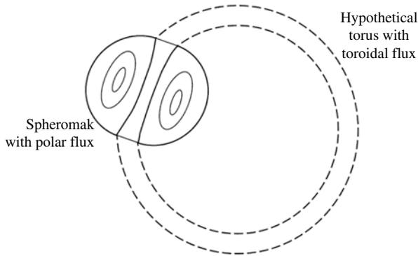
FIGURE 36. Analogy between tokamak and flux core spheromak.
