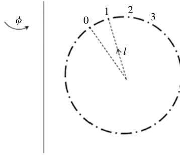
FIGURE 5. Poincaré plot generated by following a magnetic field line through many circuits around the torus.
