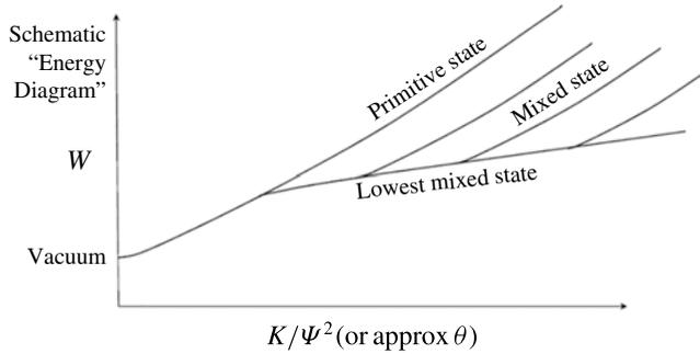
FIGURE 23. Illustration of the energy of the relaxed states in a cylindrical plasma as a function of  $K/\Psi^2$ .
