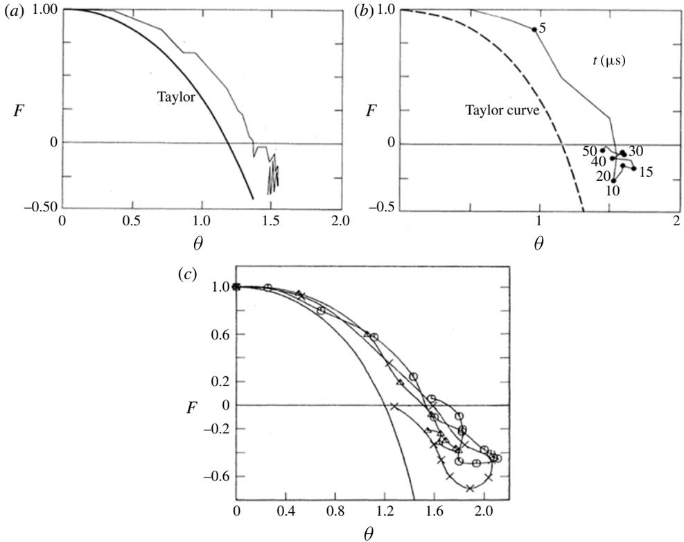
FIGURE 22. Time-dependent  $F$ - $\theta$  curves from pinches operated in slow mode: (a) ZT-40 experiment (from DiMarco 1983), (b) TPRE experiment (reproduced with permission from Tamaru *et al.* 1979) and (c) REPUTE experiment (reproduced with permission from Toyama *et al.* 1985).
