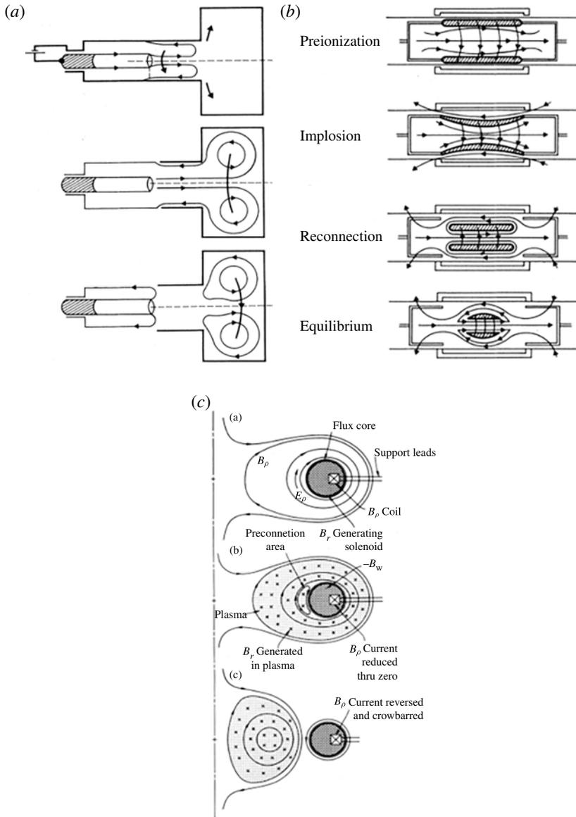
FIGURE 31. Methods to create a spheromak discharge: (a) by plasma gun (reproduced with permission from Turner *et al.* 1983, copyright 1983, AIP Publishing LLC), (b) by combined  $\theta$ - $z$  discharge (reprinted with permission from Goldenbaum *et al.* 1980, copyright 1980 by the American Physical Society) and (c) by inductive flux core in S-1 (reprinted with permission from Yamada *et al.* 1981, copyright 1981 by the American Physical Society).
