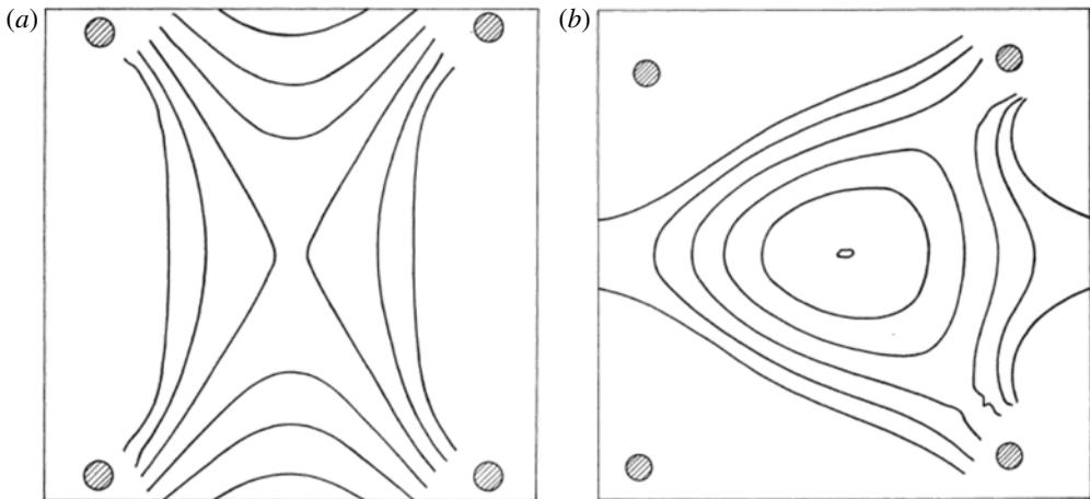
FIGURE 52. Magnetic isobars in a stabilised minimum- $B$  mirror device for (a) small current in the stabilising rods and (b) large current in the rods (from Taylor 1968).
