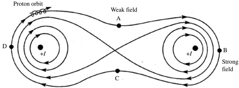
FIGURE 47. Quadrupole field configuration (from Hastie 1993).
