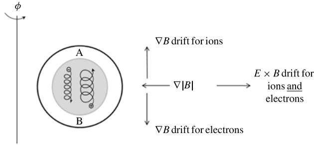
FIGURE 2. Particle motion in a toroidal field.
