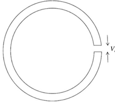
FIGURE 18. Interpreting magnetic helicity in terms of stored volt-seconds.
