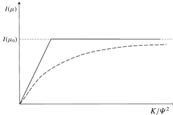
FIGURE 45. Current saturation in general relaxed states: soft (dashed) and hard (solid). Lowest eigenvalue is  $\mu_0$ .
