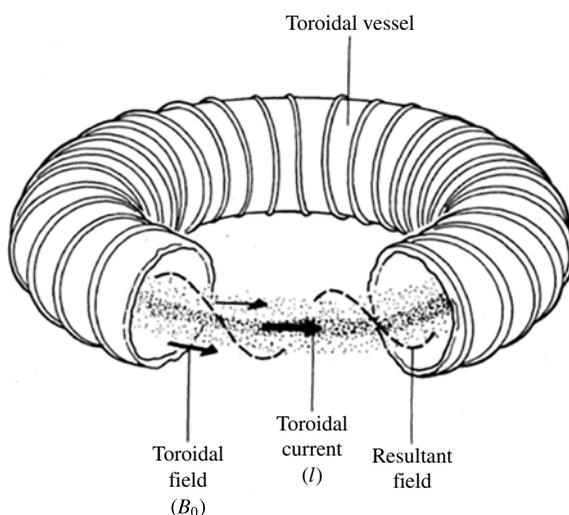
FIGURE 4. Geometry of the toroidal pinch (from Taylor 1986).
