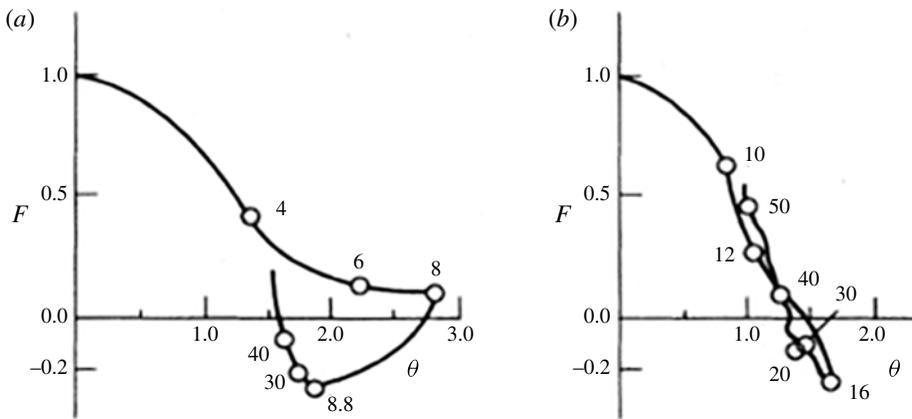
FIGURE 21. Time-dependent  $F$ - $\theta$  curve for HBTX1 in (a) fast mode and (b) slow mode. Time intervals are given in microseconds. (Reproduced with permission from Bodin & Newton (1980).)
