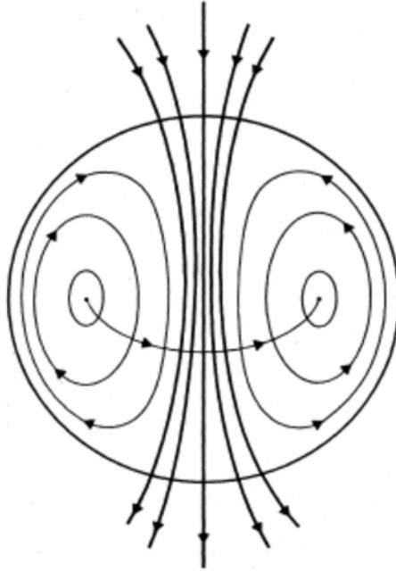
FIGURE 35. Schematic of a flux core spheromak (from Taylor 1986).
