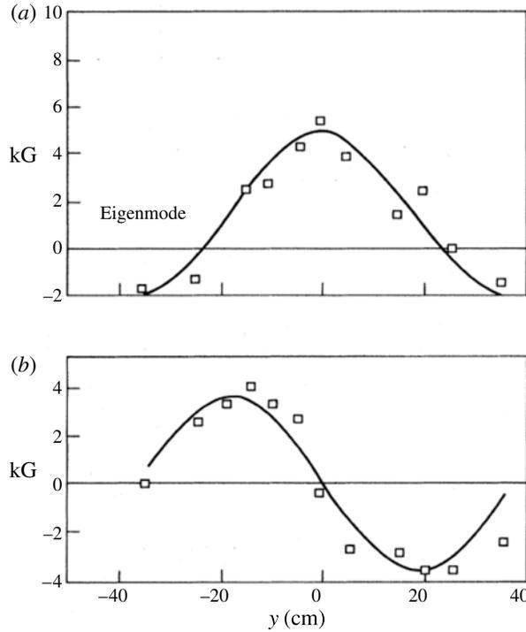
FIGURE 32. Magnetic field profiles in the BETA II spheromak. (a) Poloidal field and (b) toroidal field. Experimental measurements are shown as squares; the solid line is the theoretical prediction. (Reproduced with permission from Turner *et al.* (1983). Copyright 1983, AIP Publishing LLC.)
