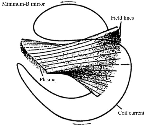
FIGURE 53. Schematic of the tennis ball coil and field lines. (Reproduced with permission from Post (1987).)
