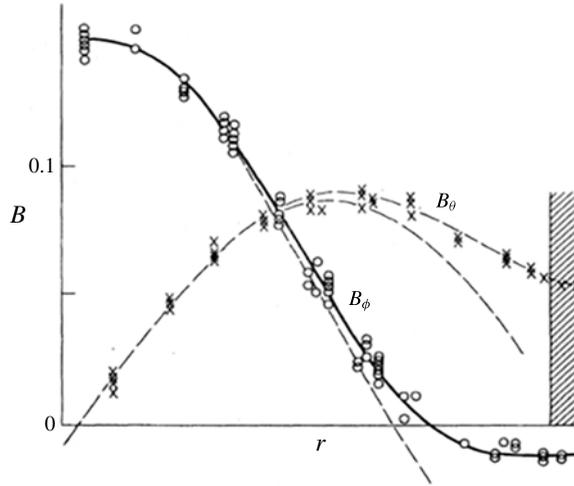
FIGURE 19. Comparison of experimental magnetic field profiles in the quiescent state of the toroidal pinch HBTX-1A to the theoretical expressions (8.4). (Reproduced with permission from Bodin (1984).)
