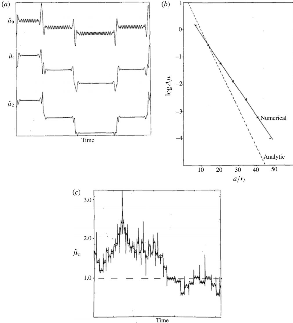
FIGURE 48. (a) Evolution of successive approximations to the particle magnetic moment as it moves in a mirror field. (b) Exponential form of the non-adiabatic jump at each transit as a function of  $a/r_L \propto 1/v$ . (c) Long-time behaviour of a non-adiabatic particle. Here  $q = 1.19$ ,  $\Phi = \pi$  and  $r/a = 0.075$ . (Reproduced with permission from Hastie *et al.* (1969).)
