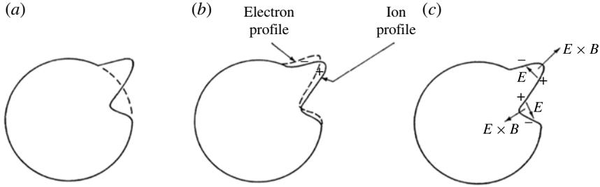
FIGURE 49. Development of the flute instability in a mirror machine (from Taylor 1968); see text for details.
