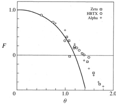
FIGURE 20. An  $F$ - $\theta$  diagram showing data from the pinch experiments HBTX1, ALPHA and ZETA and the theoretical curve. (Reproduced with permission from Bodin & Newton (1980).)
