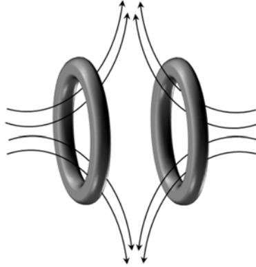
FIGURE 50. Sketch of spindle cusp configuration.
