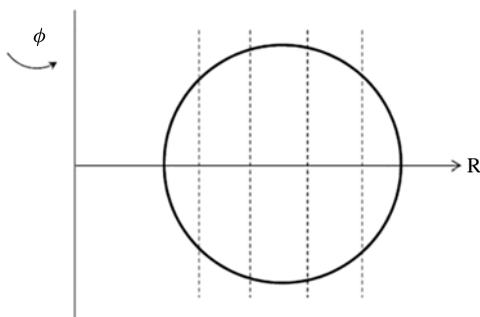
FIGURE 3. Constant pressure surfaces in a purely toroidal field.
