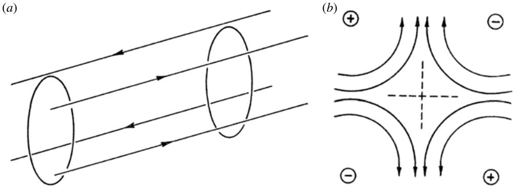
FIGURE 51. (a) Mirror machine stabilisation by Ioffe bars and (b) the resulting magnetic field (from Taylor 1968).
