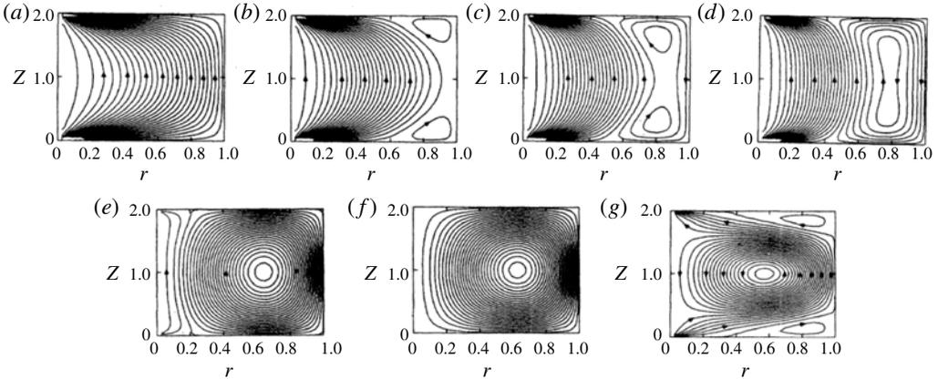
FIGURE 39. Evolution of analytic field profiles in an idealised flux core spheromak at various values of  $\mu a$ : (a)  $\mu a = 0.001$ , (b)  $\mu a = 2.25$ , (c)  $\mu a = 2.70$ , (d)  $\mu a = 3.00$ , (e)  $\mu a = 4.00$ , (f)  $\mu a = 4.14$  and (g)  $\mu a = 5.00$ . (Reproduced with permission from Turner (1984). Copyright 1984, AIP Publishing LLC.)
