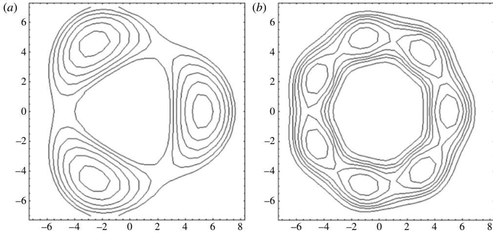
FIGURE 11. Magnetic surfaces resulting from a helical perturbation with (a)  $m = 3$  and (b)  $m = 7$ .
