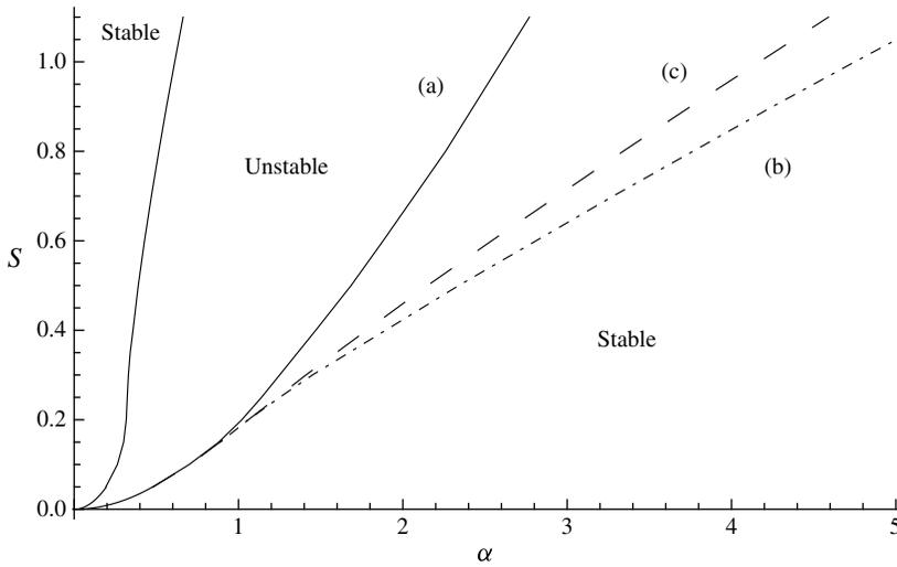
FIGURE 58. Stability boundaries for the  $s$ - $\alpha$  model obtained by taking (a)  $y_0 = 0$  (solid line), (b)  $y_0 = 0.6\pi$  (dot-dashed line) and (c)  $y_0 = \pi$  (dashed line).
