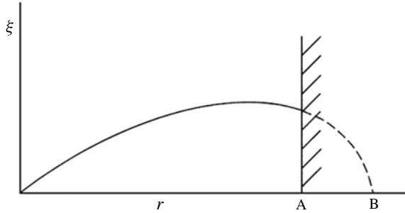
FIGURE 55. Projected displacement. A is the actual wall position and B is the hypothetical position needed for marginal stability.
