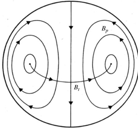
FIGURE 30. Schematic of a spheromak configuration (from Taylor 1986).
