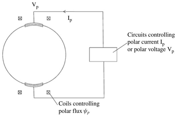
FIGURE 37. Set-up to control relaxed state of flux core spheromak externally.
