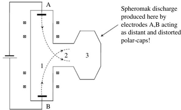
FIGURE 41. Illustration of kinked Z-pinch source.
