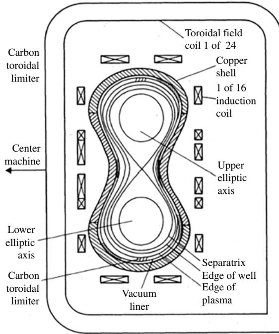
FIGURE 26. Multipinch experiment at General Atomics. (Reproduced with permission from La Haye *et al.* (1986).)
