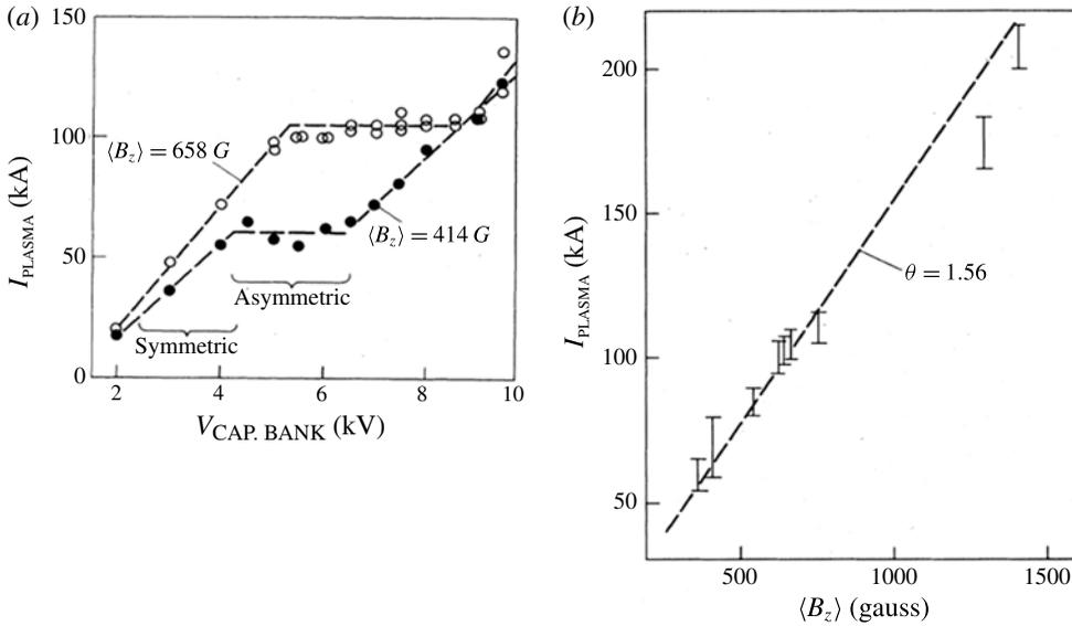
FIGURE 29. (a) Plasma current versus driving voltage and (b) variation of saturation current with toroidal flux in the multipinch. The value  $\theta = 1.56$  corresponds to  $\mu a = 2.42$  here. (Reproduced with permission from La Haye *et al.* (1986).)
