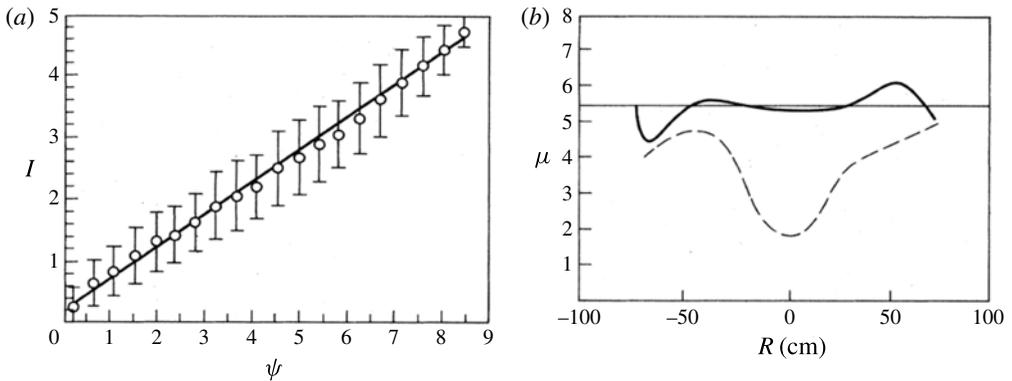
FIGURE 33. (a) Poloidal current versus poloidal flux and (b) measured profile of  $\mu(r)$  in S-1 spheromak. (Reproduced with permission from Hart *et al.* (1986). Copyright 1986, AIP Publishing LLC.)
