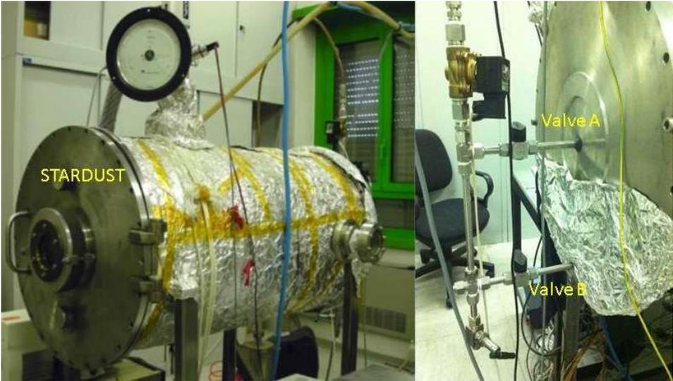
**Fig.1** STARDUST Facility (on the left) and Valves A and B (on the right) used to reproduce, LOVAs at different height
