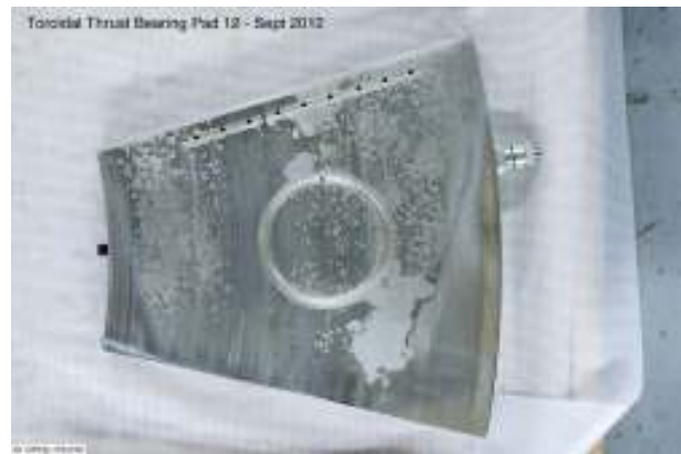
Fig 1. Pad 12 removed from the TF generator in 2012
