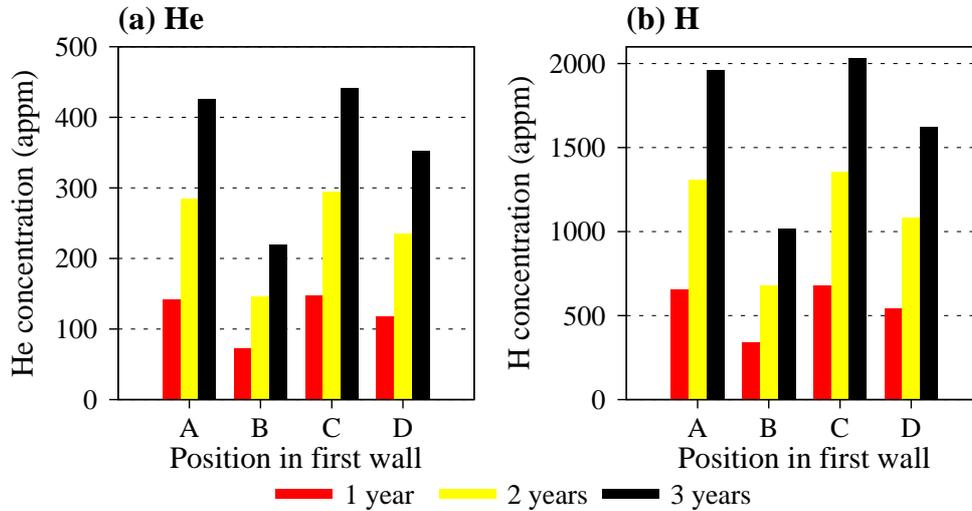
Figure 4: Variation in the (a) He, and (b) H, concentrations in pure Fe as a function of time for the spectra at different FW positions in DEMO – see figure 2.
