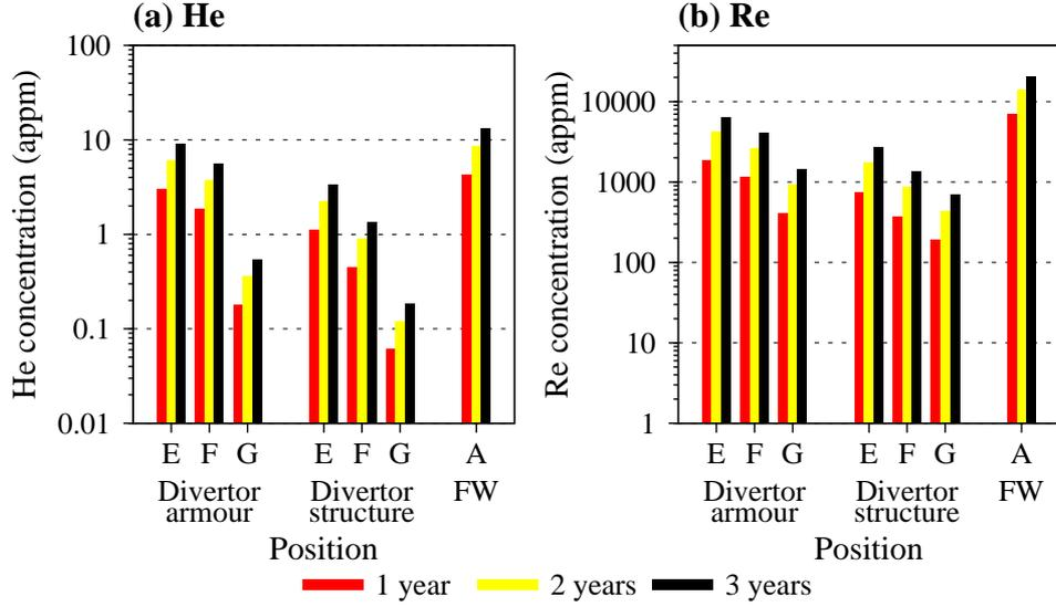
Figure 6: Variation in concentrations of (a) He, and (b) Re, produced in pure W under neutron irradiation as a function of position (and depth) in the divertor region of the DEMO design (figure 2).
