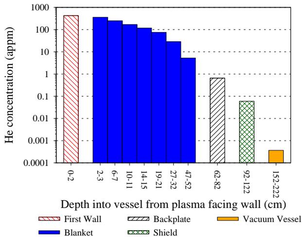
Figure 5: Variation in He concentration in pure Fe after a 3-year irradiation as a function of depth into the DEMO vessel at (A) in figure 2. Note the logarithmic scale of the concentration axes.
