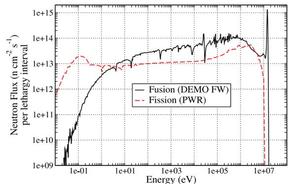
Figure 1: Comparison of the neutron-energy spectra in fission and fusion reactors. Shown is the average neutron spectrum in the fuel-assembly of a PWR reactor and the equatorial FW spectrum for the DEMO model in figure 2.
