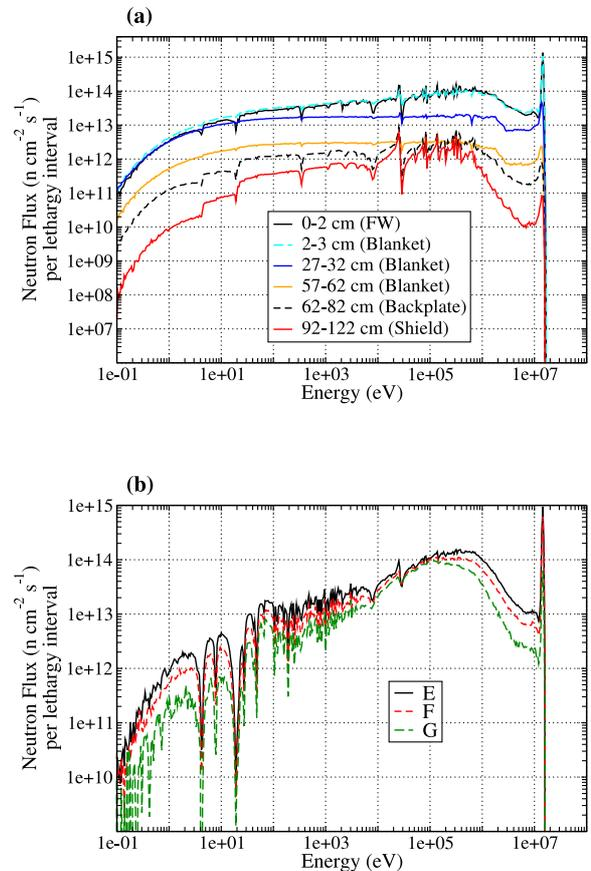
Figure 3: Comparison of the neutron-energy spectra in DEMO; (a) as a function of depth into different regions of the containment vessel at the equatorial position (A) in figure 2; and (b) in the divertor-armour layer as a function of position ((E-G) in 2)
