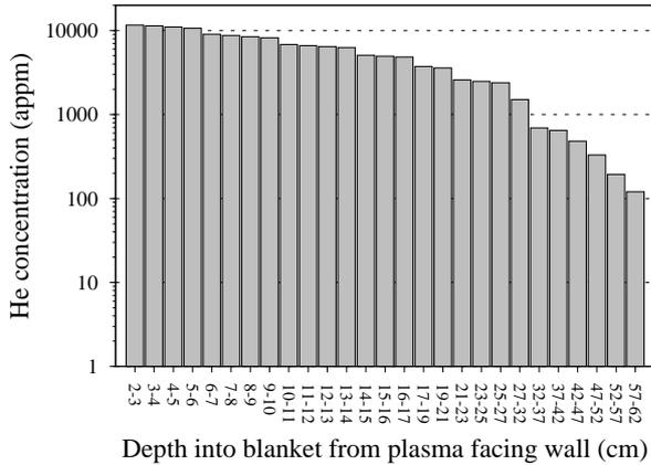
Figure 7: Variation in He concentration in pure Be after a 3-year irradiation as a function of depth into the DEMO blanket at (A) in figure 2.
