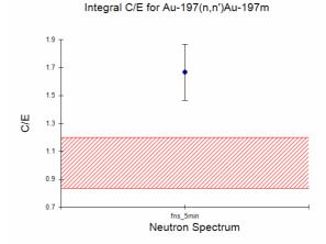
Fig. 7. C/E data for  ${}^{197}$ Au(n,n') ${}^{197m}$ Au measured in the FNS neutron spectra. The band indicates the uncertainty in the library.
