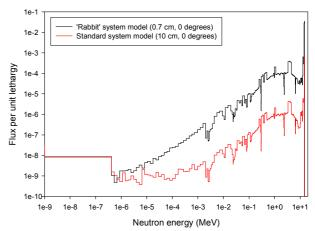
Fig. 2. Neutron spectra derived at two irradiation positions, calculated with an ASP facility model using MCNP5.
