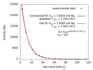
Fig. 6. Activity as a function of time for <sup>197m</sup>Au gamma line measurement at 278.99 keV for an irradiated Au foil.
