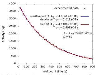
Fig. 3. Activity as a function of time for Zr-89m gamma line measurement at 587.8 keV for an irradiated Zr foil. Here and in later figures the constrained fit refers to a fit in which the half-life was fixed to the database value, while in the free fit both the half-life and  $A_0$  were allowed to vary.  $t_d$  is the time delay associated with the time between the end of the irradiation and the start of the measurement.
