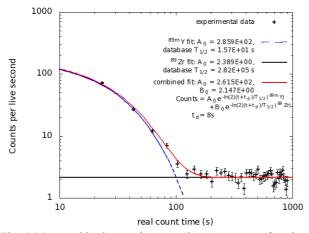
Fig. 4. Measured background corrected count rate as a function of time for the <sup>89m</sup>Y gamma line measurement at approximately 909 keV for an irradiated Zr foil.
