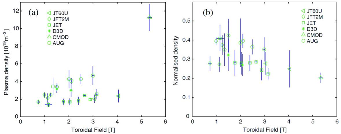
**Figure 4.** Variation of the measured minimum L–H access density (left frame) and the corresponding Greenwald fraction (right frame) with toroidal field. Reproduced with permission from [5]. © IOP Publishing.
