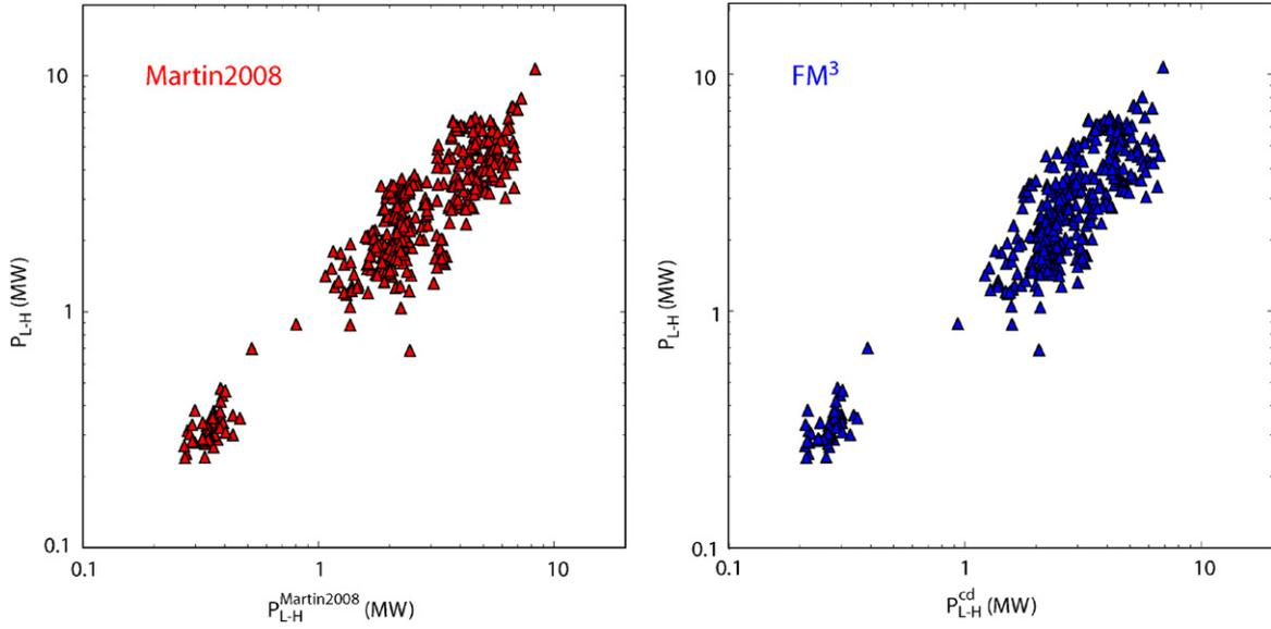
**Figure 3.** Comparison of experimental measurements of  $P_{L-H}$  on several tokamaks (ITPA data) with the best-fit scaling (left frame) (1) and the new model—labelled as  $FM^3$  after the surnames of the authors—predictions (right frame).
