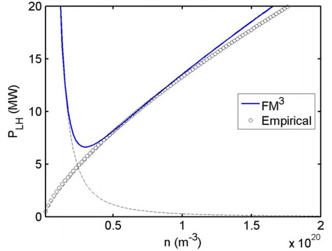
**Figure 2.** Predicted variation of  $P_{\text{L-H}}$  with plasma density for typical JET conditions. Also shown are the low and high density asymptotes, and the empirical prediction, (1).
