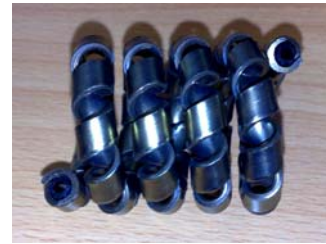
Fig. 3: Double spiral bimetallic spring
