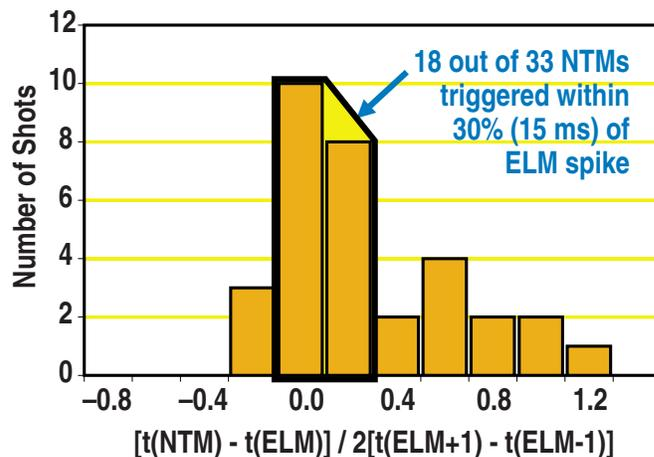
FIG. 8. (Color online) Time correlation between 2/1 NTM onset and large ELMs in DIII-D rotation scan.
