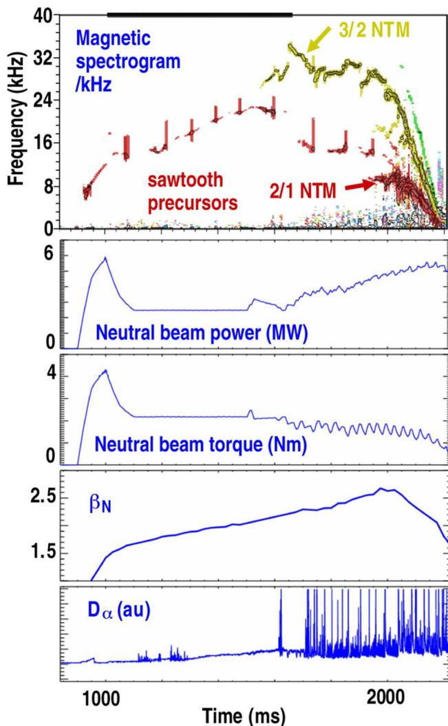
FIG. 1. (Color online) Typical shot time history (shot number 126625) showing spectrogram of Mirnov magnetic sensor, neutral beam power, and torque (smoothed to strip out modulation effects),  $\beta_N$  and  $D_\alpha$  signals.
