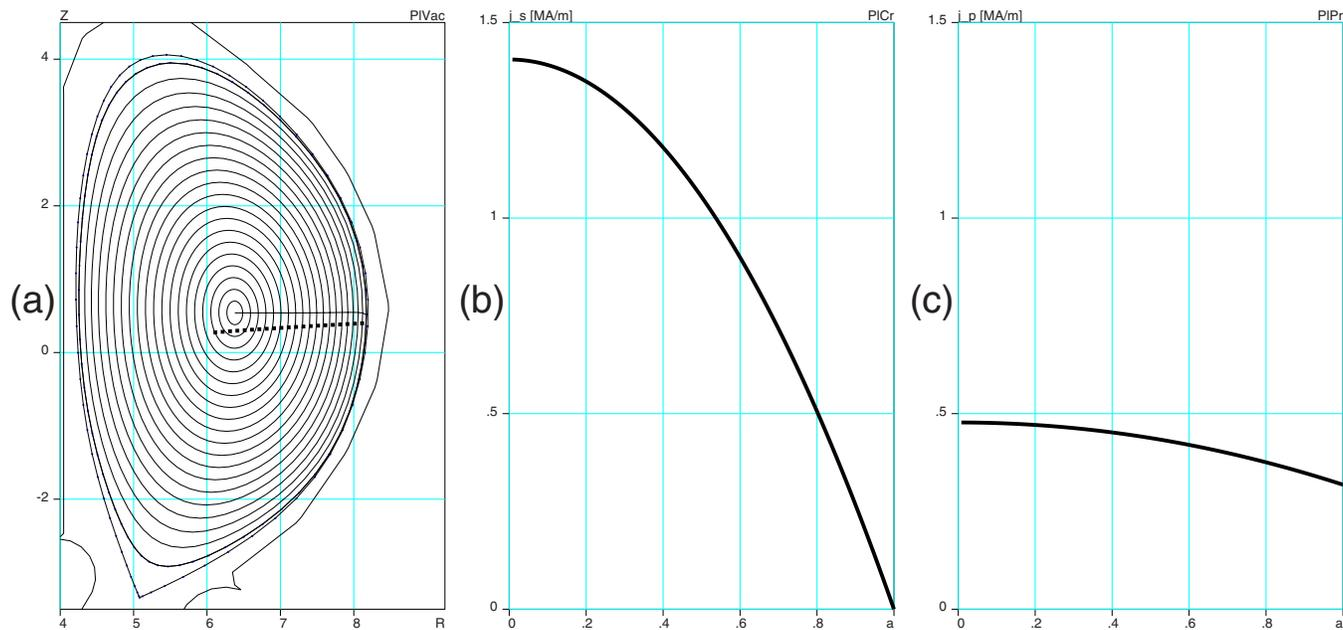
FIG. 5. (Color online) (a) Cross section of the ITER magnetic surfaces. Black dots point out the 21 MSE-LP pick-up points. (b)  $j_s$ -profile and (c)  $j_p$ -profile, which are used in equilibrium calculations.
