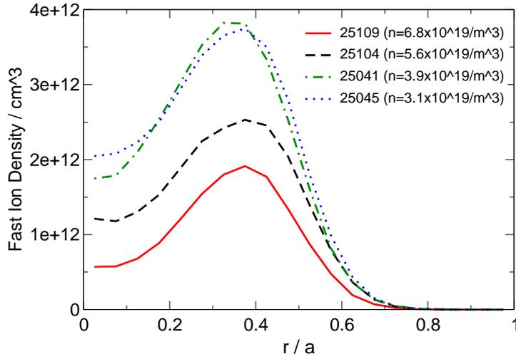
**Figure 7.** The fast ion density predicted by TRANSP as a function of  $r/a$  at  $t = 0.3s$  for four MAST plasmas, namely 25109 ( $n_e = 6.8 \times 10^{19} m^{-3}$ ), 25104 ( $n_e = 5.6 \times 10^{19} m^{-3}$ ), 25041 ( $n_e = 3.9 \times 10^{19} m^{-3}$ ) and 25045 ( $n_e = 3.1 \times 10^{19} m^{-3}$ ).
