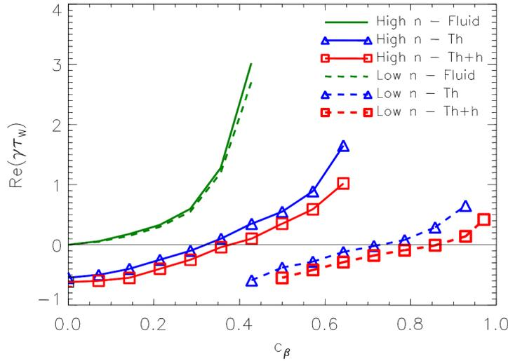
**Figure 14.** The growth/damping rate of the RWM for high and low density MAST plasmas with respect to  $c_\beta = (\beta - \beta_{nowall})/(\beta_{wall} - \beta_{nowall})$ . The damping is stronger for low density. In both cases thermal kinetic effects dominate the NBI contribution.
