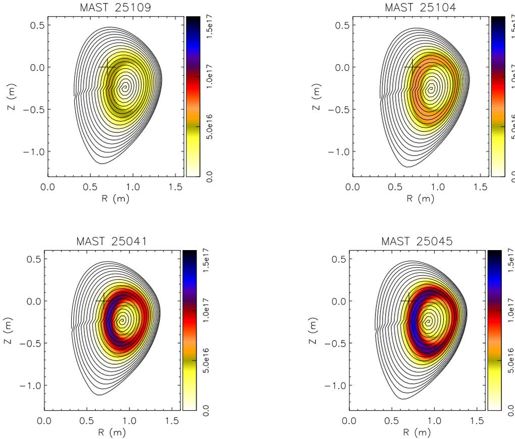
**Figure 6.** The NBI fast ion density at  $t = 0.3\text{s}$  as predicted by TRANSP for MAST discharges 25109 ( $n_e = 6.8 \times 10^{19} \text{m}^{-3}$ ), 25104 ( $n_e = 5.6 \times 10^{19} \text{m}^{-3}$ ), 25041 ( $n_e = 3.9 \times 10^{19} \text{m}^{-3}$ ) and 25045 ( $n_e = 3.1 \times 10^{19} \text{m}^{-3}$ ). As the plasma density decreases, the fast ion density increases and becomes more peaked.
