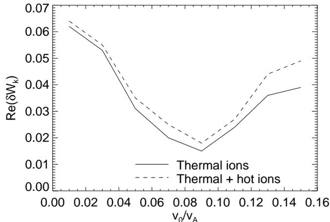
**Figure 12.** The real part of the change in the potential energy of the mode due to the kinetic response of the thermal ions and energetic beam ions with respect to the plasma frequency.
