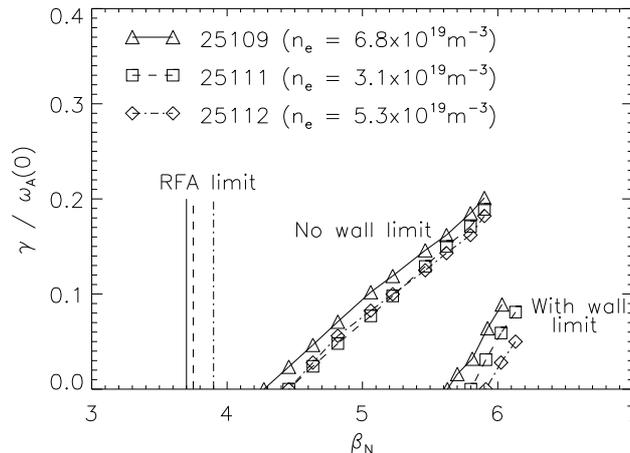
**Figure 10.** The RFA limit measured experimentally compared to the no-wall and with-wall ideal stability limits predicted by MISHKA linear stability analysis for three MAST plasmas, namely 25109 ( $n_e = 6.8 \times 10^{19} m^{-3}$ ), 25111 ( $n_e = 3.1 \times 10^{19} m^{-3}$ ) and 25112 ( $n_e = 5.3 \times 10^{19} m^{-3}$ ).
