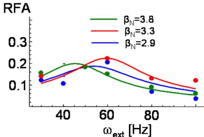
**Figure 5.** The RFA amplitude (symbols) as a function of applied field frequency for three different plasma pressures. Shown for comparison (lines) is the RFA amplitude predicted by equation 3, used to ascertain the free parameters  $\gamma_0$  and  $M_{sc}^*$ .
