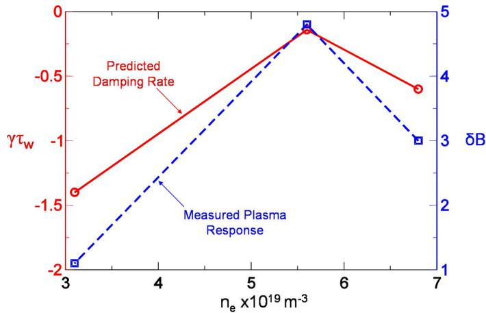
**Figure 15.** The damping rate of the resistive wall mode at  $c_\beta = 0.2$  as a function of plasma density. Also shown for comparison is the measured plasma response in the MAST shots for the same time as the equilibria used in the simulations.
