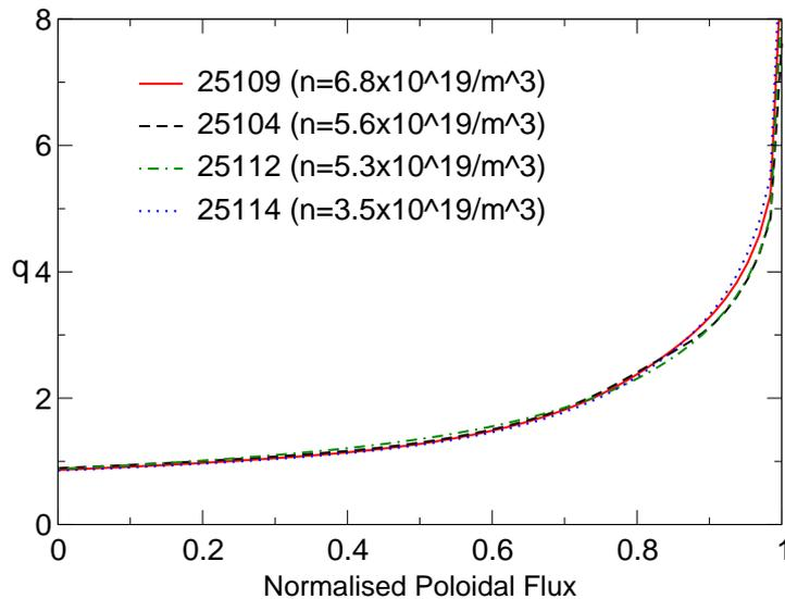
**Figure 2.** The safety factor profile at  $t = 0.3\text{s}$  for four MAST plasmas with varying plasma density, namely 25109 ( $n_e = 6.8 \times 10^{19}\text{m}^{-3}$ ), 25104 ( $n_e = 5.6 \times 10^{19}\text{m}^{-3}$ ), 25112 ( $n_e = 5.3 \times 10^{19}\text{m}^{-3}$ ) and 25114 ( $n_e = 3.5 \times 10^{19}\text{m}^{-3}$ ).
