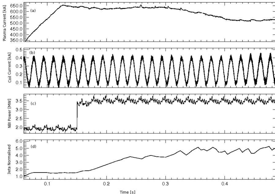
**Figure 3.** (a) The plasma current; (b) The applied oscillating field; (c) The injected NBI power and (d)  $\beta_N$  calculated by EFIT for MAST discharge 25105.
