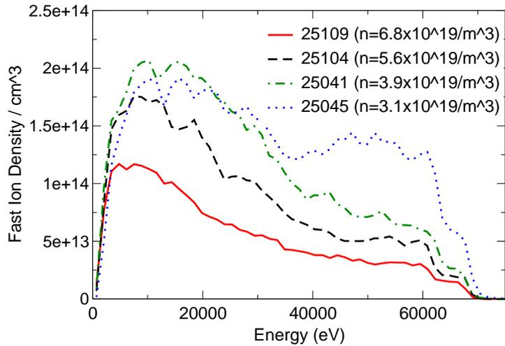
**Figure 8.** The fast ion density predicted by TRANSP as a function of particle energy at  $t = 0.3s$  for four MAST plasmas, namely 25109 ( $n_e = 6.8 \times 10^{19} m^{-3}$ ), 25104 ( $n_e = 5.6 \times 10^{19} m^{-3}$ ), 25041 ( $n_e = 3.9 \times 10^{19} m^{-3}$ ) and 25045 ( $n_e = 3.1 \times 10^{19} m^{-3}$ ).
