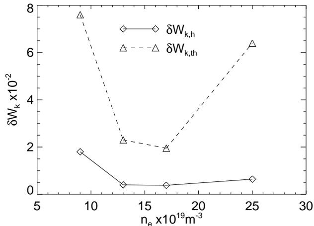
**Figure 13.** The potential energy of the mode due to the presence of energetic ions  $\delta W_{k,h}$  and thermal ions  $\delta W_{k,th}$  calculated by HAGIS for four different density MAST plasmas and respective distribution functions.
