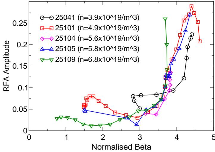
**Figure 4.** The RFA amplitude as a function of  $\beta_N$  for five MAST discharges with different plasma density, namely 25109 ( $n_e = 6.8 \times 10^{19} m^{-3}$ ), 25104 ( $n_e = 5.6 \times 10^{19} m^{-3}$ ), 25105 ( $n_e = 5.8 \times 10^{19} m^{-3}$ ), 25101 ( $n_e = 4.9 \times 10^{19} m^{-3}$ ) and 25041 ( $n_e = 3.9 \times 10^{19} m^{-3}$ ). The no-wall stability limit is taken to be where the RFA begins to markedly increase as the mode approaches marginal stability.
