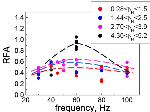
**Figure 1.** The resonant field amplification amplitude as a function of applied oscillating field frequency. It is apparent that the clearest amplification is observed when the applied field is at 60Hz.
