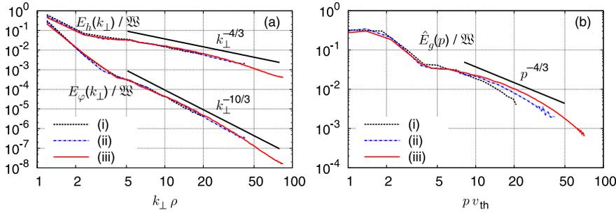
FIG. 3 (color online). Time-averaged normalized (a) wave-number (Fourier) spectra  $E_h(k_\perp)/2B$  and  $E_\varphi(k_\perp)/2B$  [cf. (9)], and (b) velocity-space (Hankel) spectrum  $\hat{E}_g(p)/2B$  for the runs indexed in Table I. Theoretically predicted slopes are given for comparison.
