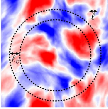
FIG. 1 (color online). Schematic view of the nonlinear phase mixing superimposed on the potential from the Run (iii) (see Table I) at  $t/\tau_{\text{init}} = 10$  and the largest wavelength mode taken out. When the fluctuation scale  $\ell \lesssim \rho$ , the gyroaverage of the electric field induces a decorrelation of the distribution function at the velocity-space scale corresponding to the difference in Larmor radii  $\ell_v = \delta v/\Omega \sim \ell$  [see (7)].
