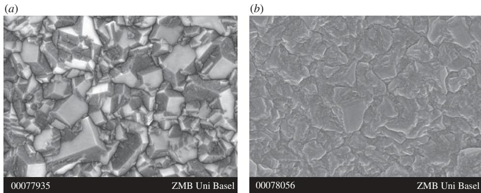
Figure 2. Scanning electron microscopy micrographs of a microcrystalline chemical vapour deposition (CVD) diamond film on a Mo substrate (Heriot-Watt University) (a) before and (b) after exposure to a high-density H plasma in the Pilot PSI plasma simulator. The surface grains are rounded and eroded but overall the coating was not heavily affected. Scale bars, (a,b) 500 nm.
