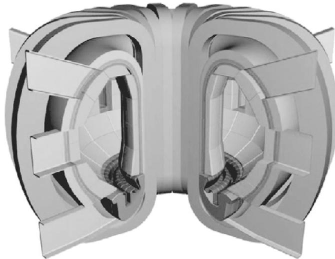
Figure 1. Schematic representation of a fusion power plant design. The superconducting magnets are the outer layer. The vacuum vessel, the first wall and the blanket are inside the vacuum vessel and the dark region round the base of the tokamak represents the divertor.
