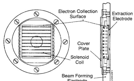
FIG. 5. The variable magnetic field suppressor.
