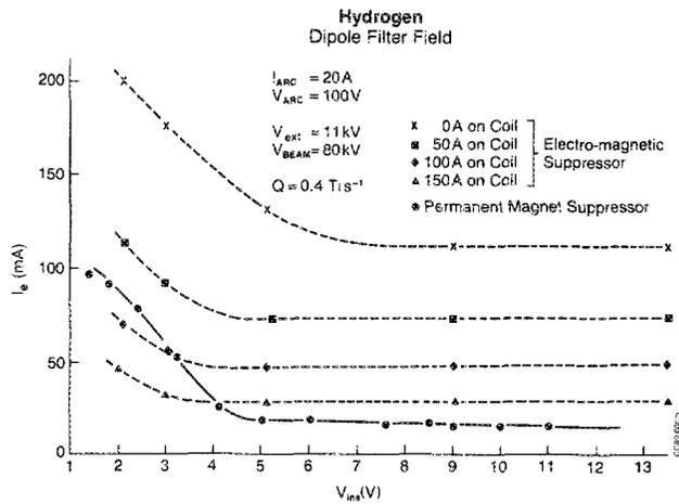
FIG. 6. The suppression of electrons at  $I_{ARC} = 20$  A.
