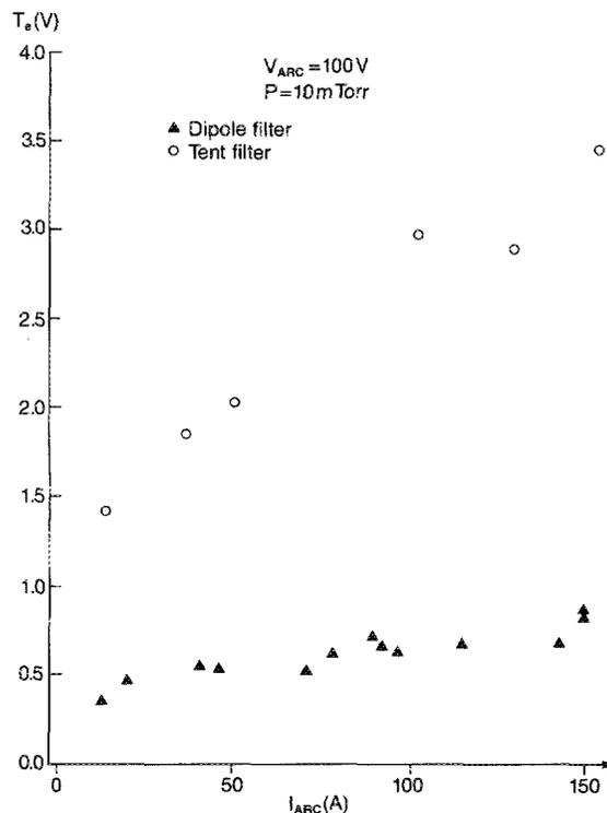
FIG. 11. The dependence of electron temperature on arc current for the source filter configurations.
