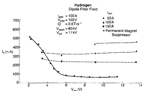
FIG. 7. The suppression of electrons at  $I_{ARC} = 100$  A.
