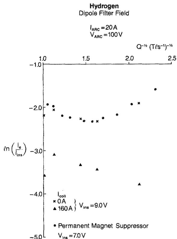
FIG. 16. The variation of  $\ln(I_e/I_{ins})$  vs  $Q^{1/2}$  ( $Q \propto$  pressure) for the two suppressor.
