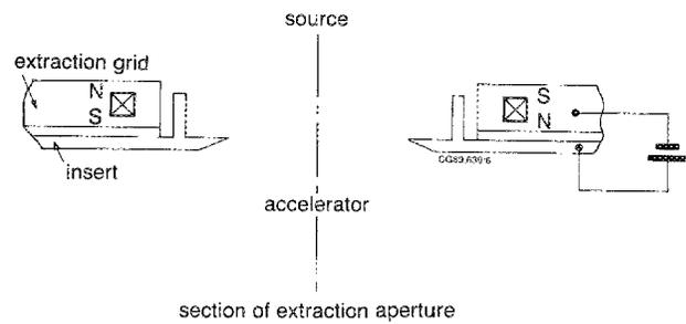
FIG. 4. The permanent magnet electron suppressor.
