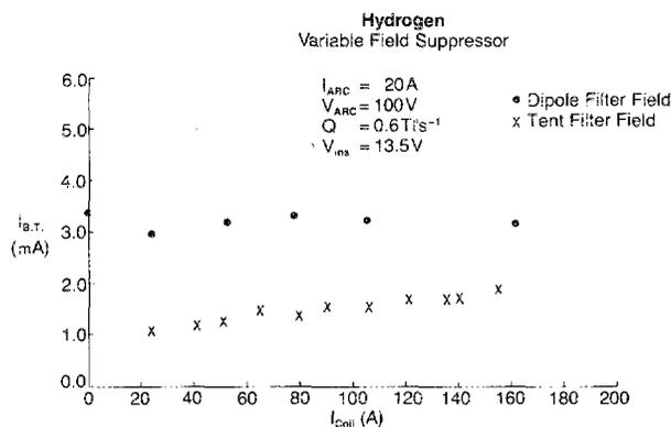
FIG. 10. The dependence of the extracted negative ion current on the magnetic field from the electromagnetic suppressor for both the dipole and tent source filter configurations.
