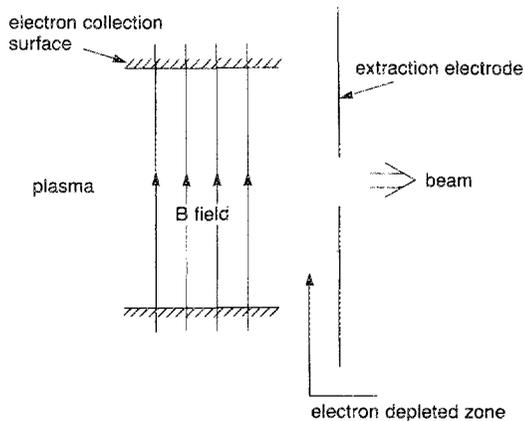
FIG. 3. Schematic of the electron suppressor.
