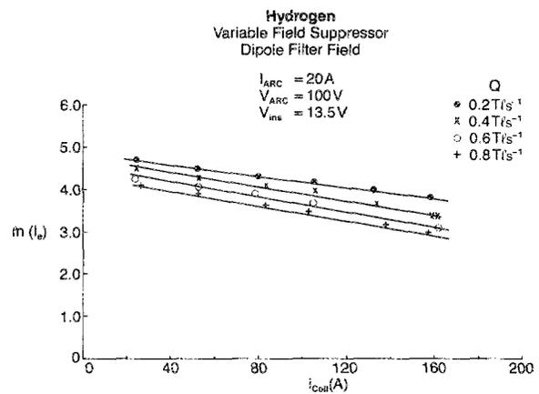
FIG. 13. The variation of extracted electron current on the magnetic field for the electromagnetic suppressor.
