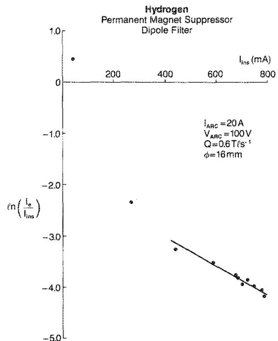
FIG. 14. The variation of  $\ln(I_e/I_{ins})$  vs  $I_{ins}$  for the permanent magnet suppressor.
