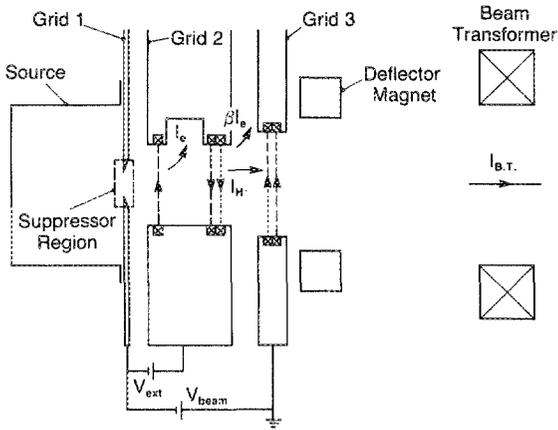
FIG. 2. The source and accelerator.
