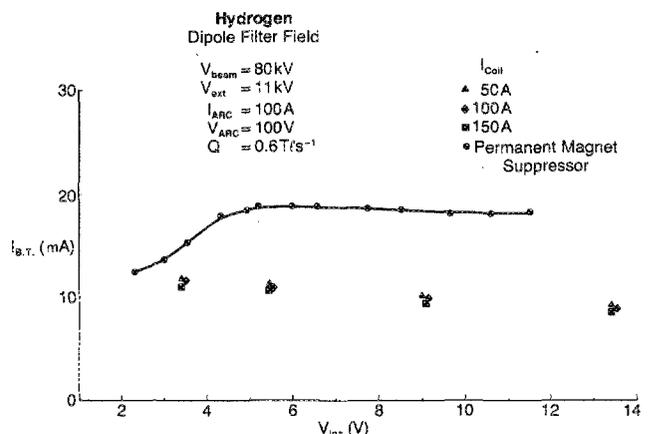
FIG. 9. The effect of electron suppression on the extracted negative ion current at  $I_{ARC} = 100$  A.
