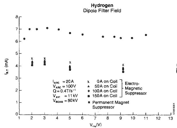
FIG. 8. The effect of electron suppression on the extracted negative ion current at  $I_{ARC} = 20$  A.
