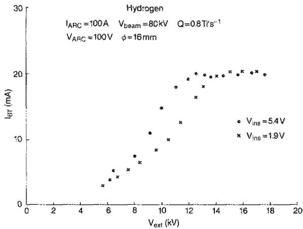
FIG. 12. Variation of transported ion current with extraction voltage for different values of suppressor voltage.
