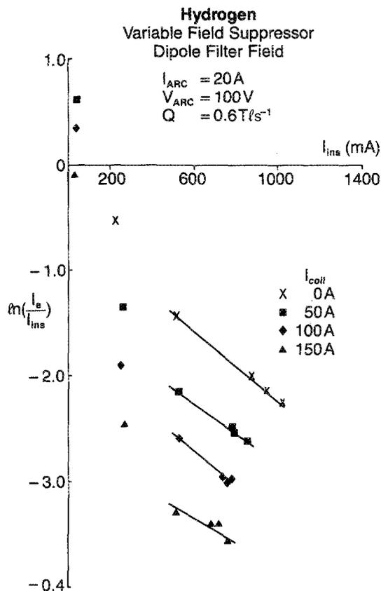
FIG. 15. The variation of  $\ln(I_e/I_{ins})$  vs  $I_{ins}$  for the electromagnetic suppressor.
