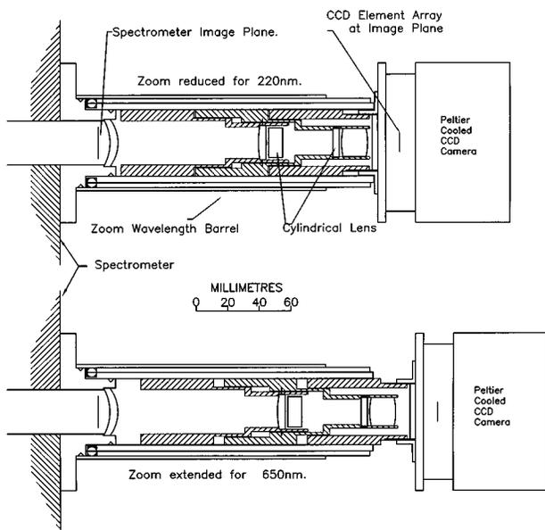
FIG. 3. Anamorphic lens that couples the dispersed spectra to the CCD detector array. Cylindrical lens elements are used to achieve the unequal vertical and horizontal (spectral) magnification. A zoom-wavelength system is also incorporated.
