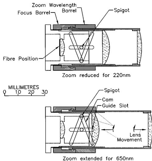
FIG. 1. Collection lens with short and long wavelength settings. When the zoom-wavelength barrel is rotated it moves the lenses by distances determined by the pitch of the cams on the lens tubes.
