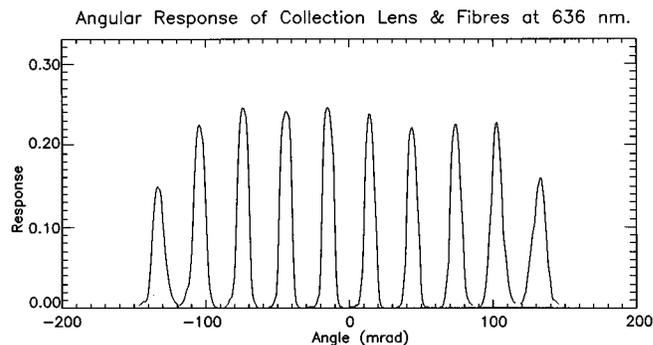
FIG. 2. Relative response curves of the ten fiber bundles,  $4 \times 400 \mu\text{m}$  diameter, from one of the  $f/2$  15° field-of-view collection lenses.
