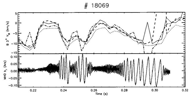
FIG. 4. Comparison of Doppler  $B^{3+}$  (282 nm)  $V_\phi$  velocities from four chords on COMPASS-D and the MHD radial magnetic field,  $b_r$ , waveform in the presence of a magnetic island.
