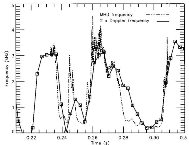
FIG. 5. The data from one of the chords and the  $b_r$  waveform in Fig. 4 are here compared in terms of toroidal frequency.
