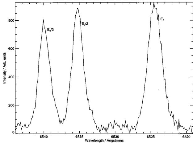
FIG. 6. Doppler shifted  $H_{\alpha}$  spectrum arising from the  $E_0$ ,  $E_0/2$ , and  $E_0/3$  energy components measured from the neutral beam atoms on the START device.
