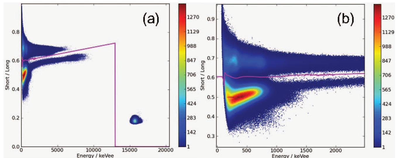
FIG. 4. KM12 heating phase PSD of  $5.7 \times 10^7$  events (a) and a detail (b) showing the separation line (magenta) for  $n/\gamma$  discrimination using tomographic analysis.
