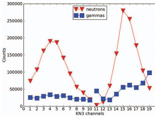
FIG. 16. Profile of neutron and gamma counts KN3 measured during the NBI steady phase of shot 83 550.
