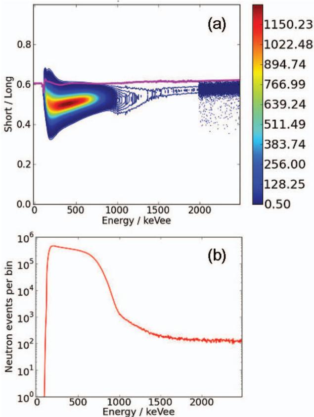
FIG. 6. Tomographic reconstructed KM12 neutron PSD for the heating phase of JET experimental campaigns C28-C30 ( $4.1 \times 10^7$  events). In (a), the neutron contribution into the gamma region is visible above the  $n/\gamma$  separation line (magenta) with  $R = 0.2\%$ . The color scale is relative to model amplitudes. In (b), the corresponding neutron pulse height spectrum as a projection of the neutron PSD onto the energy axis in log scale.
