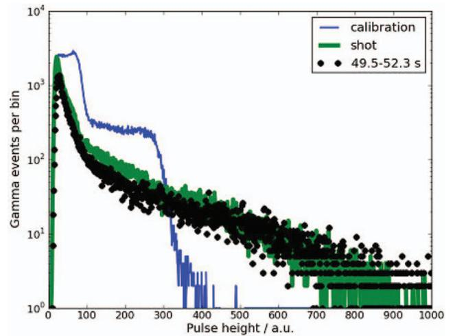
FIG. 17. KN3 channel 15 gamma pulse height spectra measured during the calibration, the shot and for 2.8 s of the NBI steady phase of shot 83 550.
