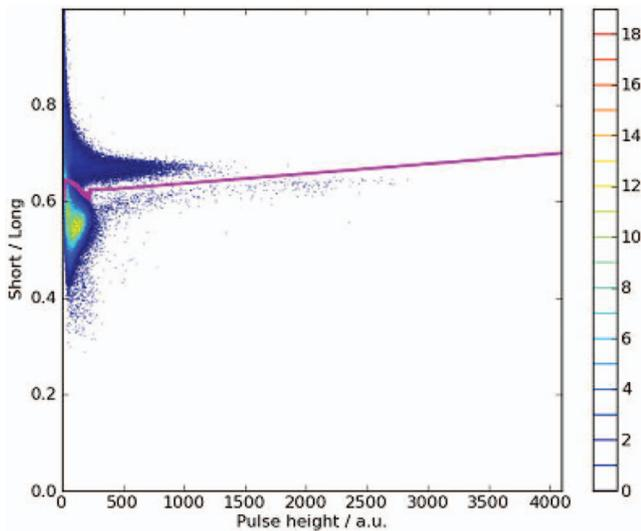
FIG. 12. KN3 channel 15 PSD of shot 83 550 during 49.5–52.3 s of NBI steady phase. The total number of events is  $3.4 \times 10^5$ .
