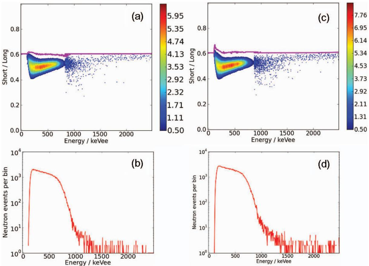
FIG. 11. Tomographic reconstructed KM12 neutron PSD for shot 83 550 (a) extracted from the PSD displayed in Figure 9(a). The color scale is relative to model amplitudes. In (b), the corresponding neutron pulse height spectrum in log scale. Panels (c) and (d) display similar results for shot 83 551 (Figure 9(b)).
