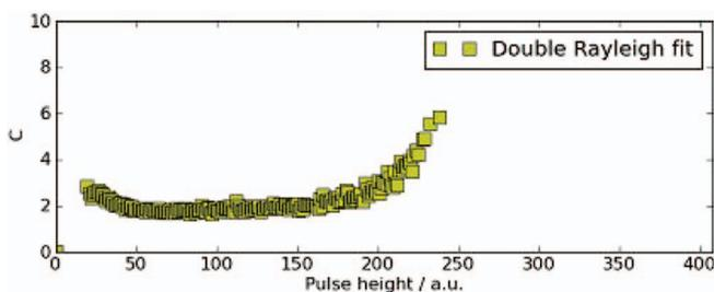
FIG. 13. KN3 channel 15 results of Double Rayleigh model comparison in terms of Cash statistics  $C$  for shot 83 550 during the NBI steady phase (49.5–52.3 s).
