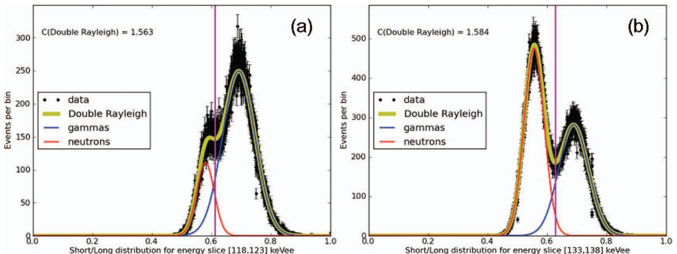
FIG. 2. Short/Long distributions obtained from the PSD shown in Figure 1 for radiation energy deposited about 120 keVee and 135 keVee. They are compared to the Double Rayleigh model (yellow line) in terms of Cash statistics  $C$ . The magenta vertical line corresponds to the local minimum of model and it is used as  $n/\gamma$  separation point in that specific PSD slice. The red and blue lines represent the individual Rayleigh distribution of the neutron and gamma lobes.
