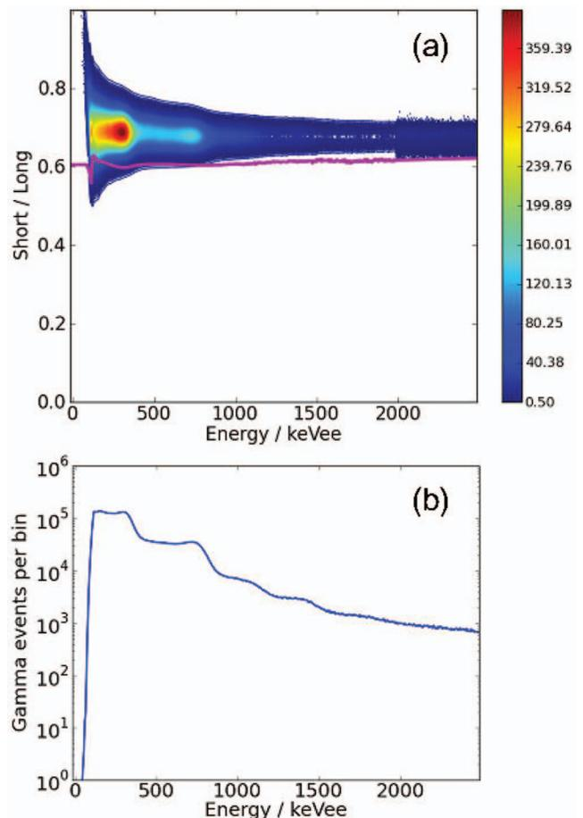
FIG. 7. As Figure 6 but for gammas ( $1.1 \times 10^7$  events) where  $R = 1.9\%$  are identified as being in the neutron region.
