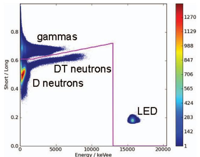
FIG. 1. KM12 PSD distribution of Short/Long gates vs. radiation deposited energy (proportional to the Total gate) obtained for just the heating phase of all shots of JET experimental campaign C28–C30 ( $5.7 \times 10^7$  events). The magenta  $n/\gamma$  separation line is defined visually.<sup>8</sup>
