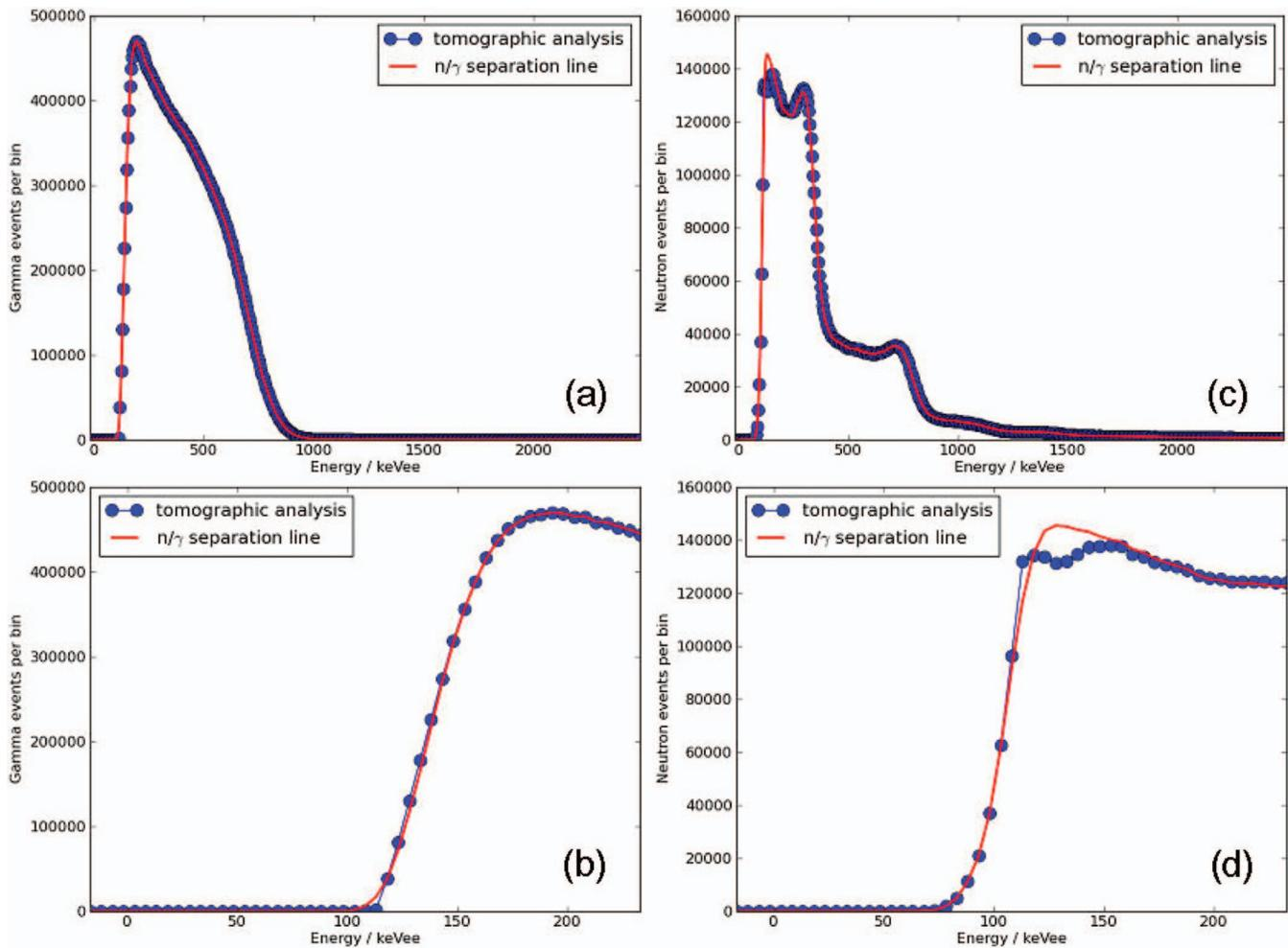
FIG. 8. Comparison of the neutron (a) and gamma (c) pulse height spectra of the heating phase PSD (Figure 4(a)) obtained using the tomographic analysis and the  $n/\gamma$  separation line of Figure 1. A magnification of the spectra low energy region is shown in panels (b) and (d), respectively.
