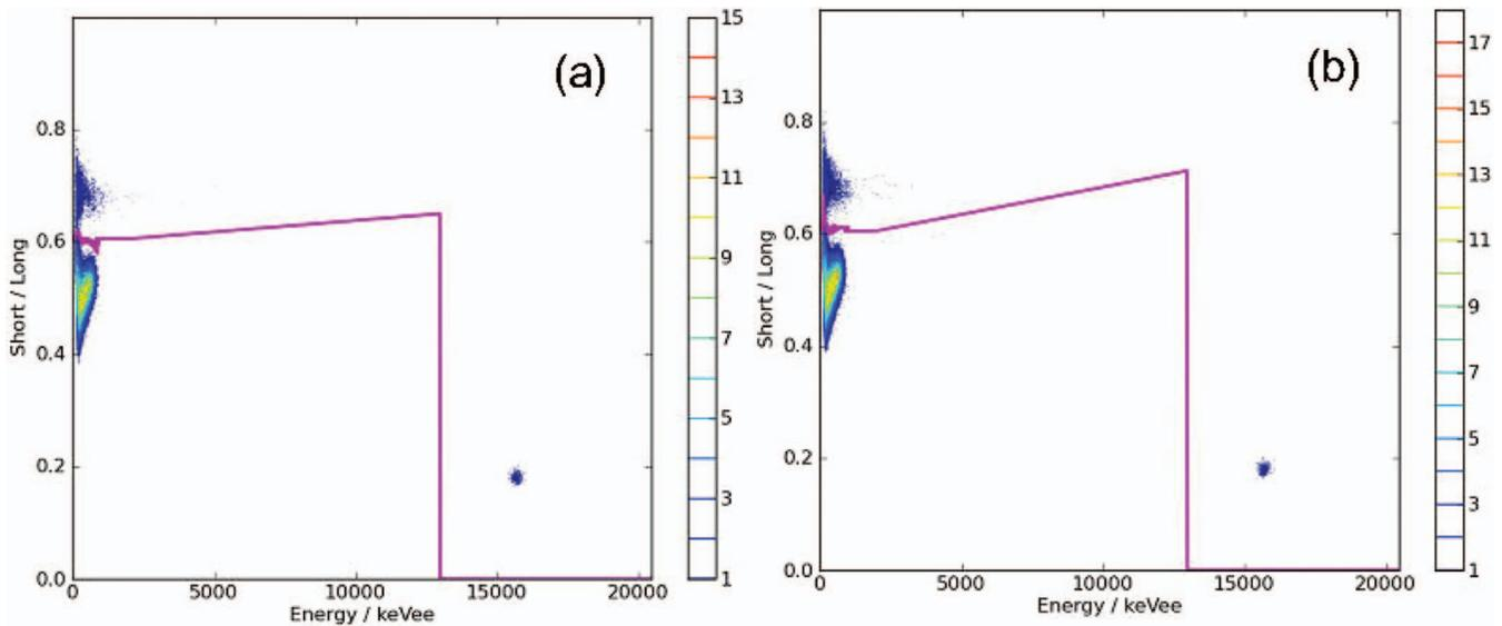
FIG. 9. PSD of shots 83 550 (a) and 83 551 (b) during 49.5–52.3 s of NBI steady phase. The total number of events is  $2.0 \times 10^5$  and  $2.7 \times 10^5$ , respectively, of which  $3.0 \times 10^3$  are due to the LED control and monitoring system.
