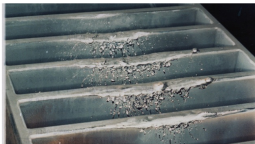
Figure 2. RE-induced damage of a stainless steel antenna from 1983 ASDEX experiments on lower hybrid heating [53, 54] due to \geq 5 MeV electrons that also caused nuclear material activation. Courtesy of Dr F. Leuterer with permission.
