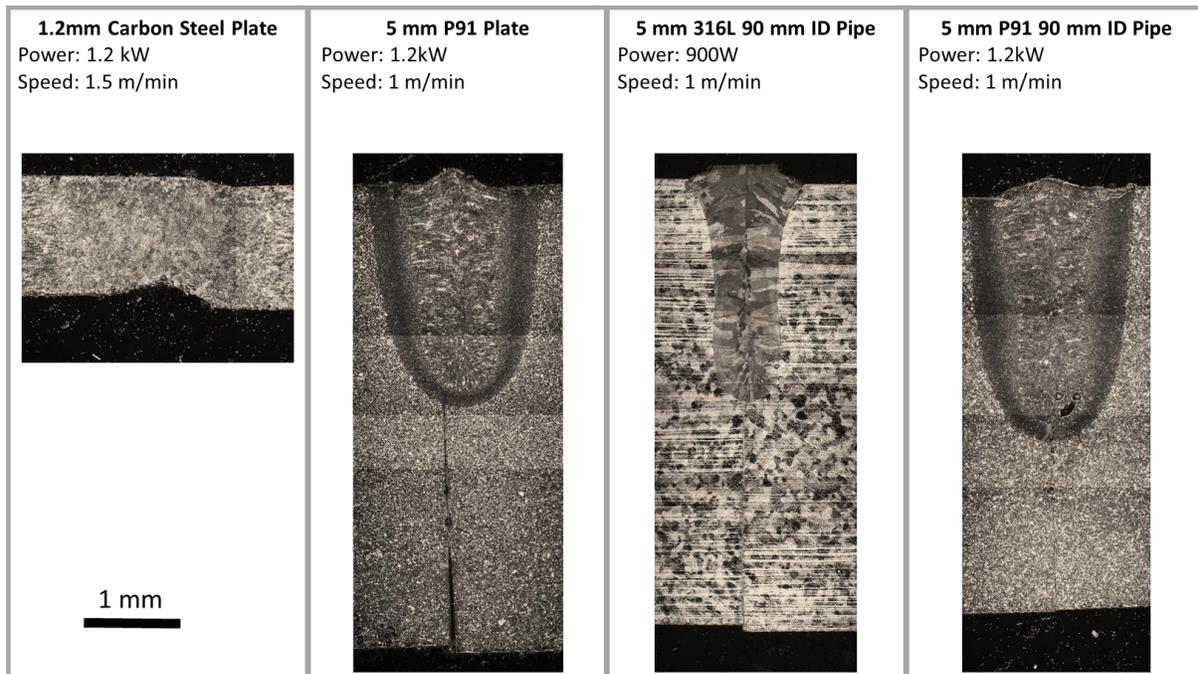
Fig. 6. Cross-sections of welds produced by the miniaturised laser welding head. The notes above each cross-section lists the process conditions and material sample.
