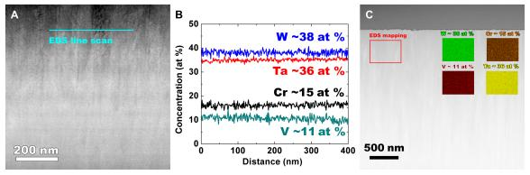
Fig. 1. Alloy composition. (A) Cross-sectional transmission electron microscopy (TEM) image of the HEA film showing a region where EDS line scan is performed. (B) EDS line scan concentration profiles of the elements in the HEA film. (C) Cross-sectional scanning electron microscopy micrograph with EDS maps of the elemental composition on the HEA film.
