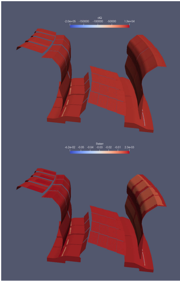
Fig. 10. Absolute (top) and relative error (below) in power deposition due to failure of flux conservation along a fieldline. runid = 271.1-fsdfia-fiar.
