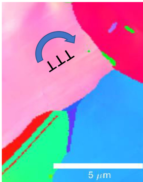
Fig. 2. Illustration of the lattice rotation about the dislocation line direction in a pileup.
