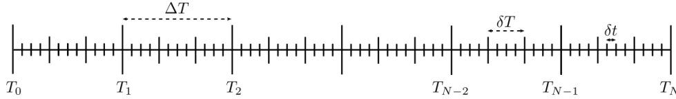
FIG. 1. Schematic of the time domain decomposition. Three levels of temporal discretisation are shown: subintervals (size \Delta T ), coarse intervals (size \delta T ), and fine intervals (size \delta t ). Note how the discretizations align with one another and that \delta t \ll \delta T \leq \Delta T in our implementation.
