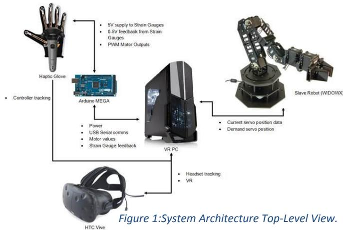
Figure 1: System Architecture Top-Level View.
