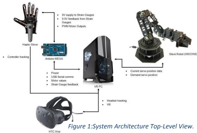
Figure 1: System Architecture Top-Level View.
