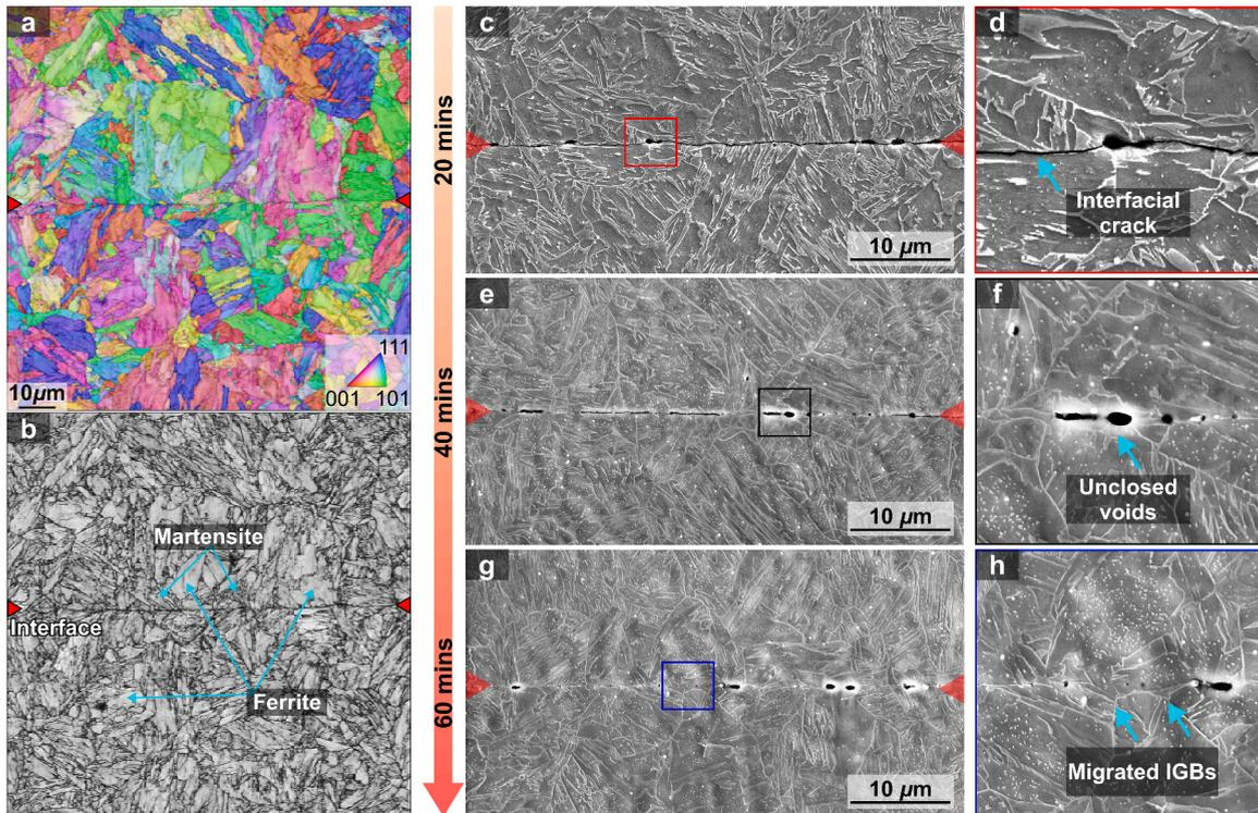
**Fig. 2.** Microstructure details of as-bonded 9Cr-1Mo steel after diffusion bonding at 900 °C: (a) EBSD-IPF map after 20 mins bonding, (b) EBSD-BC map after 20mins bonding, (c) and (d) SEM images after 20 mins bonding, (e) and (f) SEM images after 40 mins bonding, (g) and (h) SEM images after 60 mins bonding.
