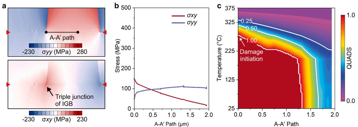
Fig. 7. IGB behaviours in the case without void: (a) normal  $\sigma_{yy}$  and shear stress  $\sigma_{xy}$  at the temperature where damage initiates, (b) line results of normal  $\sigma_{yy}$  and shear stress  $\sigma_{xy}$  at the same temperature of (a), (c) QUADS distribution along with IGB with the change of temperature.
