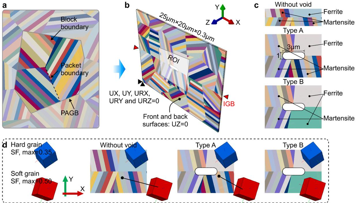
**Fig. 5. Details of representative volume:** (a) hierarchical structure of martensite, (b) boundary conditions and ROI, (c) three cases with different local microstructure in ROI, (d) orientation control in three cases.
