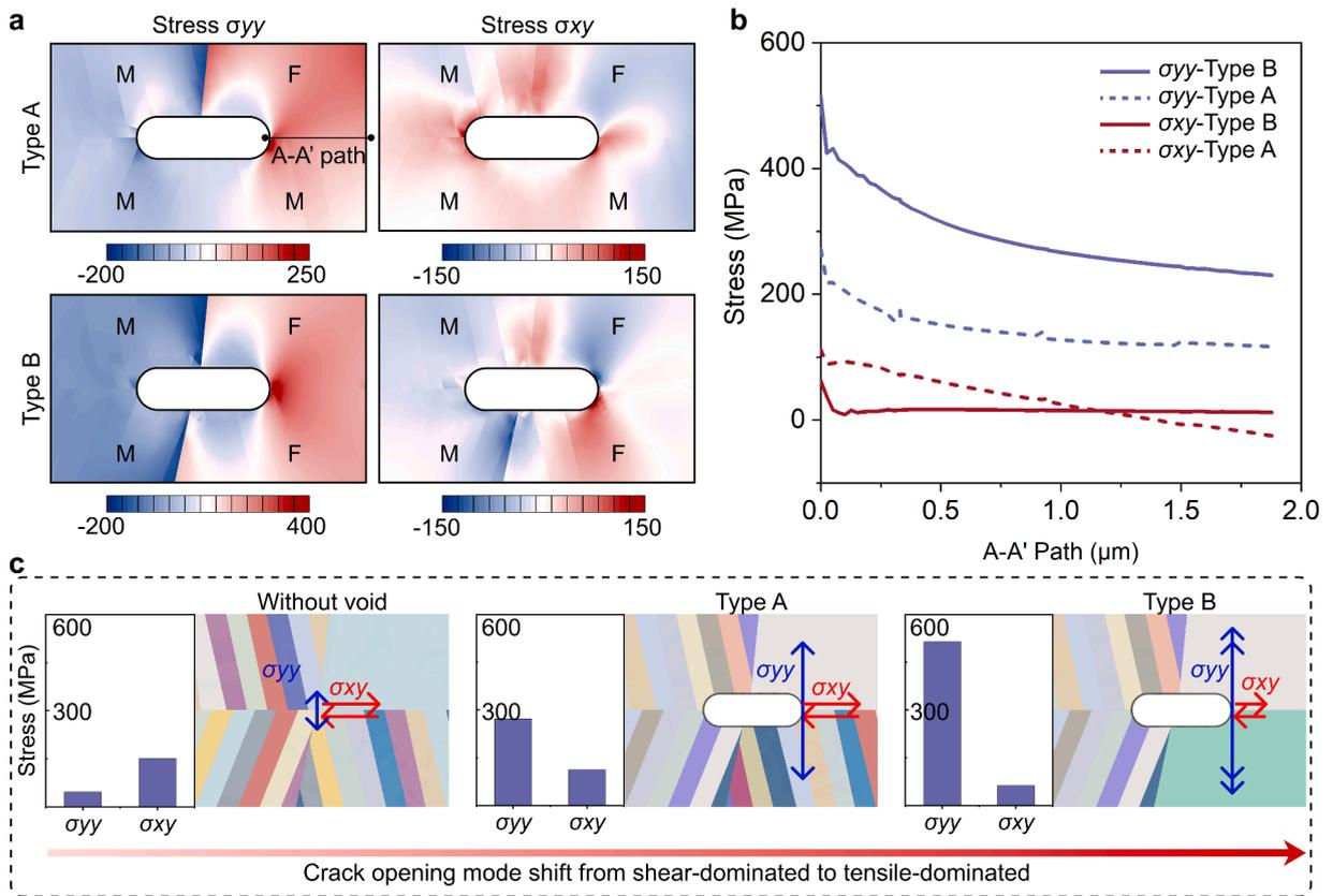
Fig. 9. Stress state at IGB during cooling: (a) distributions of  $\sigma_{yy}$  and  $\sigma_{xy}$  in Type A and B at 280 °C, (b) line results in path A-A' according to Fig. 9a, (c) summary of stress opening mode for the cases without void and Types A and B with voids.
