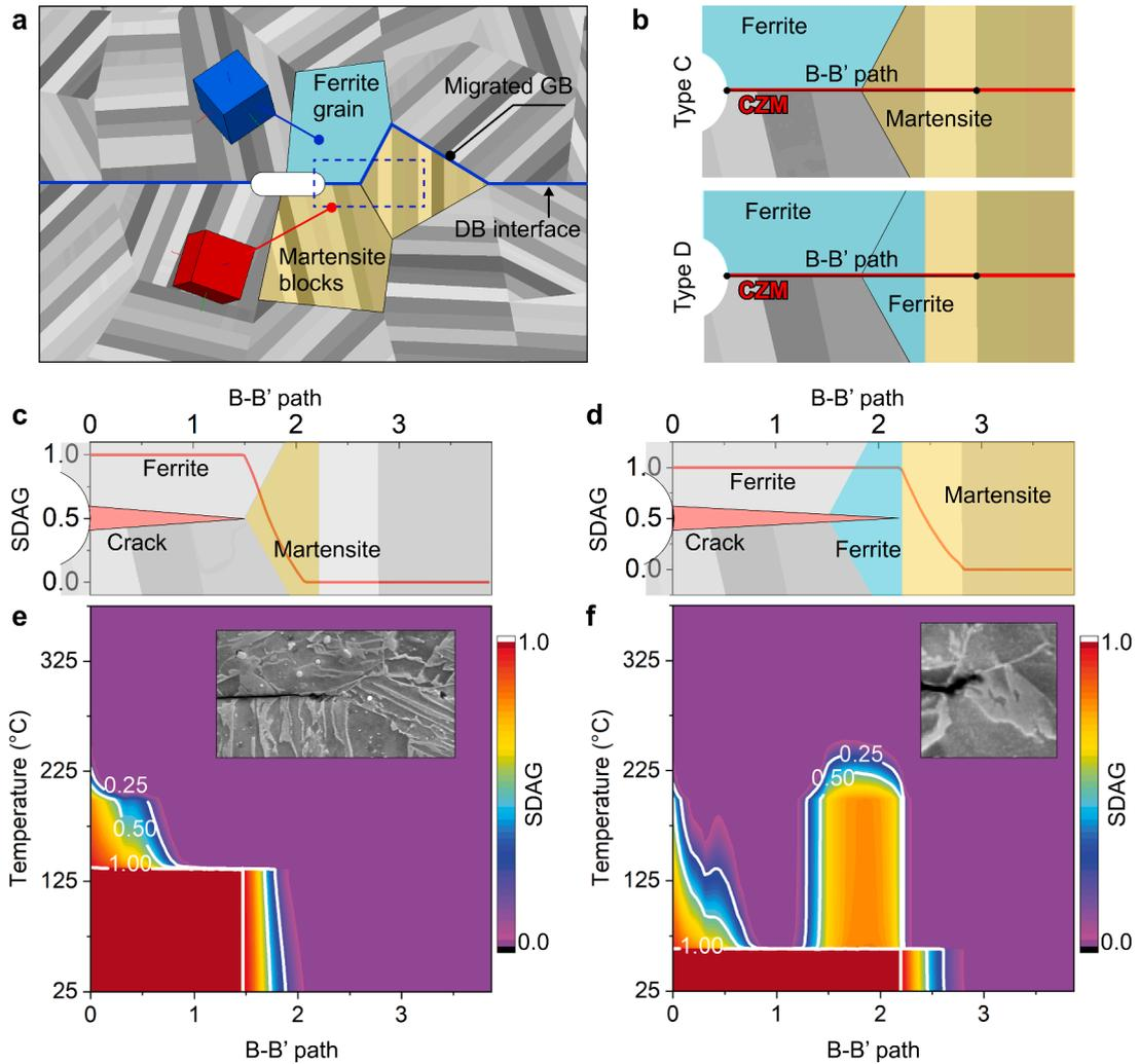
**Fig. 12. Model details and cracking behaviours considering the IGB migration:** (a) grain morphology, (b) two types with different phase distribution, (c) SDAG of Type C after cooling with phase distribution overlaid, (d) SDAG of Type D after cooling, (e) SDAG evolution of Type C, (f) SDAG evolution of Type D.
