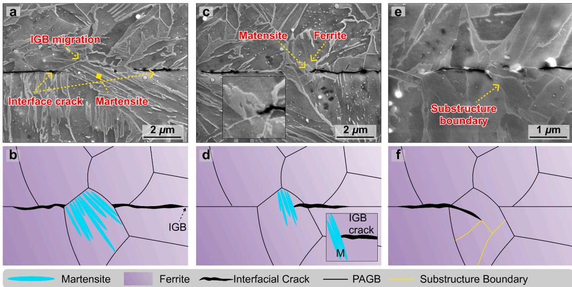
**Fig. 11. Three microstructure features with respect to the effects of IGB migration on interfacial cracking:** (a) and (b) show crack propagation stopping when it encountered a migrated IGB with martensite, (c) and (d) show the crack path through the ferrite but stopping in front of the martensite, (e) and (f) shows the crack following the substructure boundary of grain.
