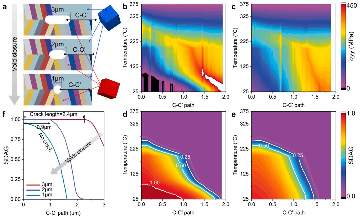
**Fig. 14.** Effects of void closure on IGB cracking: (a) models with three lengths of voids, (b) evolution of  $\sigma_{yy}$  with 2 $\mu\text{m}$  void, (c) evolution of  $\sigma_{yy}$  with 1 $\mu\text{m}$  void, (d) evolution of SDAG with 2 $\mu\text{m}$  void, (e) evolution of SDAG with 1 $\mu\text{m}$  void, (f) comparison of SDAG obtained after the cooling process among three models.
