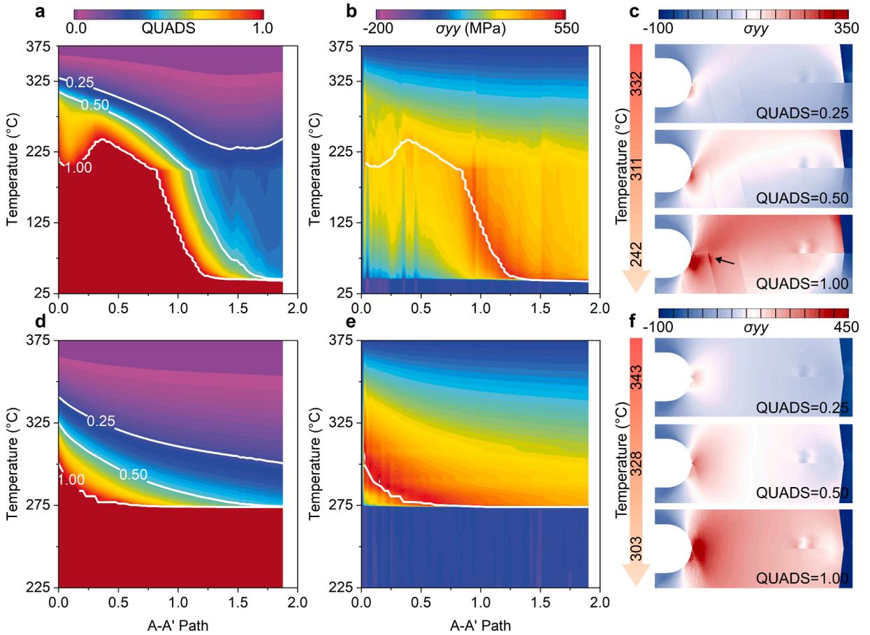
**Fig. 10. Relationship between IGB damage behaviours and stress:** (a) and (d) show evolutions of QUADS; (b) and (e) are evolutions of  $\sigma_{yy}$ , (c) and (f) are distributions of  $\sigma_{yy}$  at three typical moments. (a), (b) and (c) are results of Type A; (d), (e) and (f) are results of Type B.
