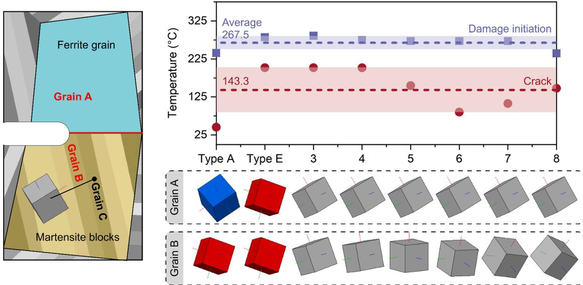
Fig. 17. Crystallographic sensitivity of IGB damaging and cracking.
