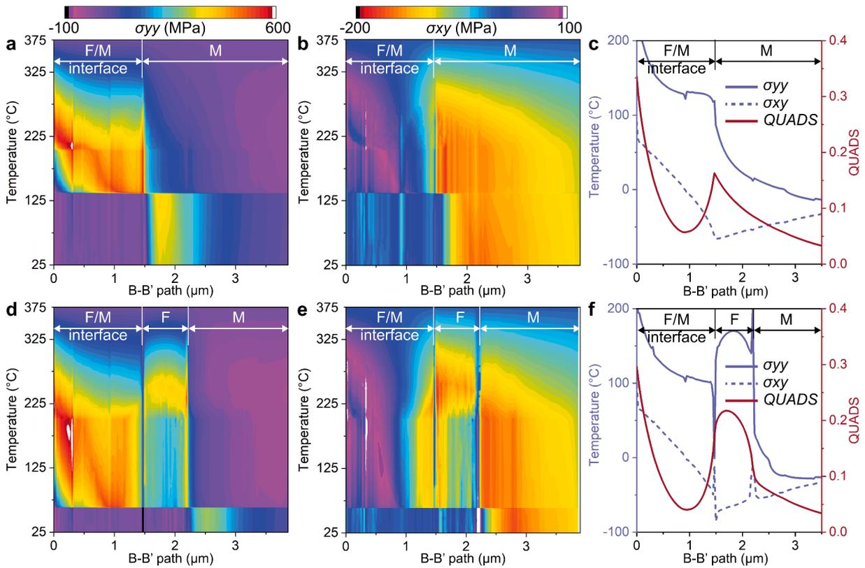
**Fig. 13. Evolution of stress components and IGB damage with respect to the effects of IGB migration:** (a) and (b)  $\sigma_{yy}$  and  $\sigma_{xy}$  in Type C, (c) line results of  $\sigma_{yy}$ ,  $\sigma_{xy}$  and QUADS in Type C, (d) and (e)  $\sigma_{yy}$  and  $\sigma_{xy}$  in Type D, (f) line results of  $\sigma_{yy}$ ,  $\sigma_{xy}$  and QUADS in Type D.
