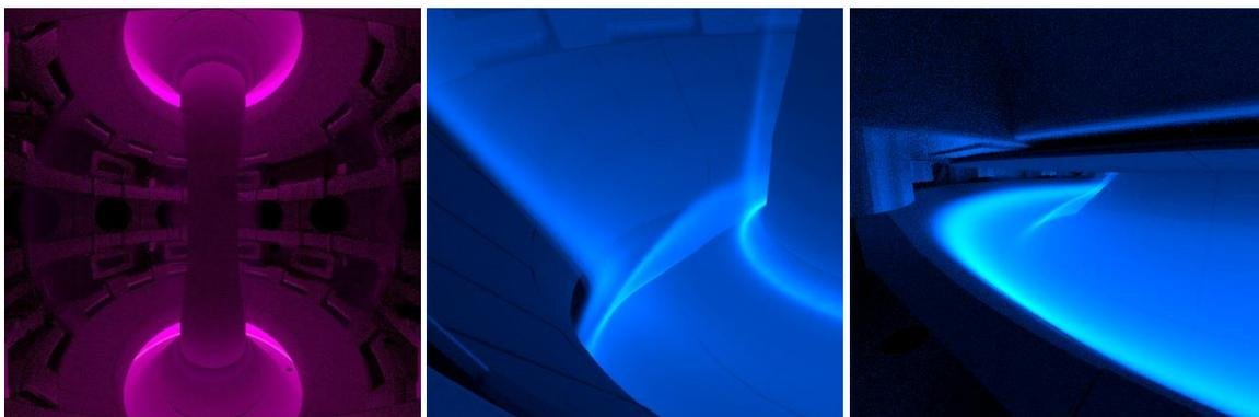
Figure 9: Synthetic camera images of emission from neutral deuterium (left) and  $C^{2+}$  ions calculated from a SOLPS simulation of MAST Upgrade as viewed from filtered cameras installed to monitor the lower X-point and inner divertor (middle) and lower divertor chamber (right).
