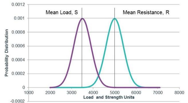
Figure 1: Example Load and Resistance Probability Density Graph
