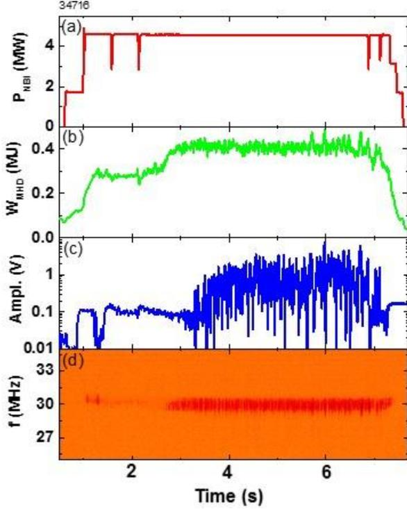
FIG. 2. A “classic” ICE example of low field side edge emission due to NBI fast ions on ASDEX Upgrade (discharge #34716,  $B_T = -2.47$  T,  $H^+$  plasma,  $H^+$  beams). The plotted quantities are (a) the NBI power  $P_{\text{NBI}}$ ; (b) the stored plasma energy  $W_{\text{MHD}}$ ; (c) the RF probe amplitude on the low field side, on a logarithmic scale; and (d) the measured ICE intensity frequency spectrum  $f$ , on a logarithmic scale (see (c) for relative scale).
