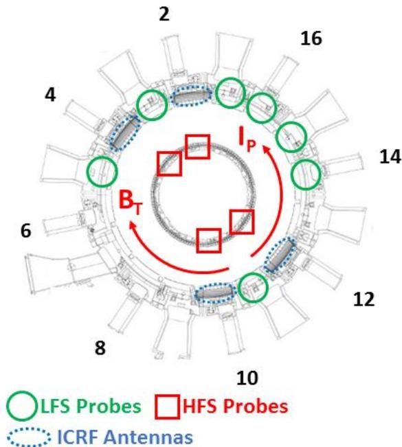
FIG. 1. The top cross-sectional view of the RF probe positions in ASDEX Upgrade. Shown are the low field side (LFS) probes, the high field side (HFS) probes, and the ICRF antennas. The standard direction of the plasma current  $I_P$  (+) and the toroidal magnetic field  $B_T$  (-) are shown. The numbers indicate the torus sector locations (only even numbers are shown).
