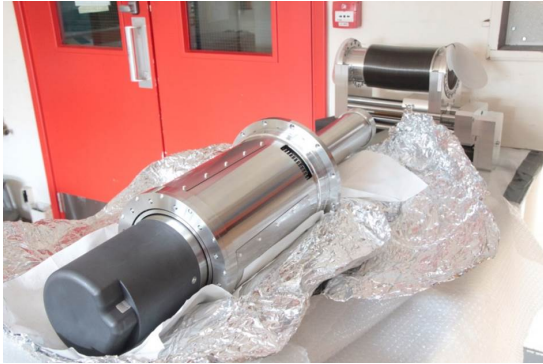
FIG. 6. Picture of the assembled MAST-U FILD.
