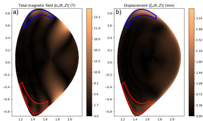
Figure 1: The peeling response typically manifests as a peak in the total field and displacement near the plasma X point and top, where the poloidal field is minimised. Data from 33353 at 2.325s. a)  $b_nT$  and  $b_nX$  are the maximum total magnetic field within the blue and red solid lines respectively. b)  $\xi_nT$  and  $\xi_nX$  are the maximum plasma displacement within the blue and red solid lines respectively.
