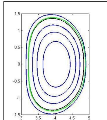
Figure 3: Tokamak geometry showing the saturated fluxtube, in green. The blue line denote the flux surfaces in the plasma
