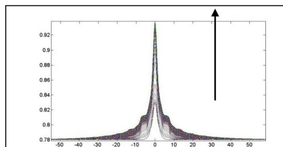
Figure 4: The evolution of a flux tube with time under viscous drag. Horizontal axis is distance along the field line. Vertical axis is the minor radius. The displacement is localized around the outboard midplane. The unstable flux displacement saturates.
