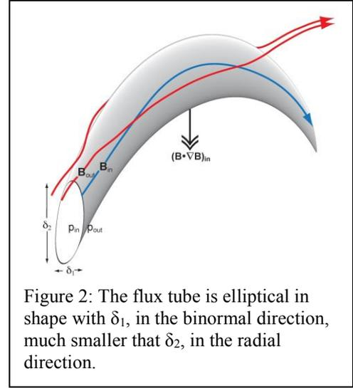
Figure 2: The flux tube is elliptical in shape with  $\delta_1$ , in the binormal direction, much smaller than  $\delta_2$ , in the radial direction.
