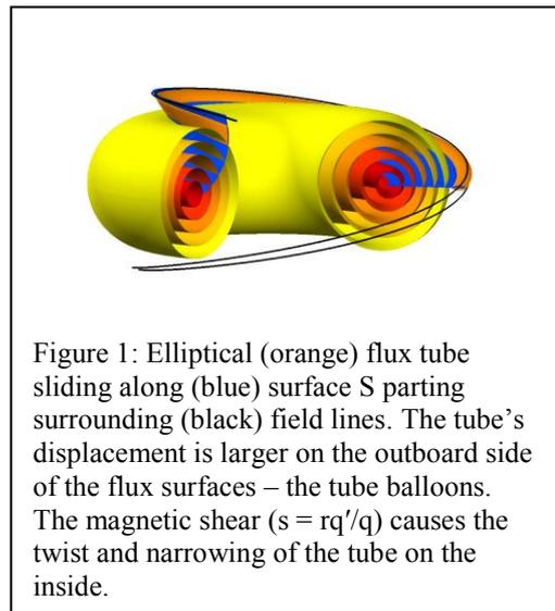
Figure 1: Elliptical (orange) flux tube sliding along (blue) surface  $S$  parting surrounding (black) field lines. The tube's displacement is larger on the outboard side of the flux surfaces – the tube balloons. The magnetic shear ( $s = rq'/q$ ) causes the twist and narrowing of the tube on the inside.
