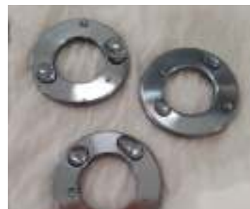
Fig. 3. CHEF Friction Disks During Soak Test (MoST)
