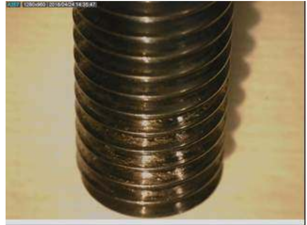
Fig. 9. MoST Coating Damage After 6 Cycles
