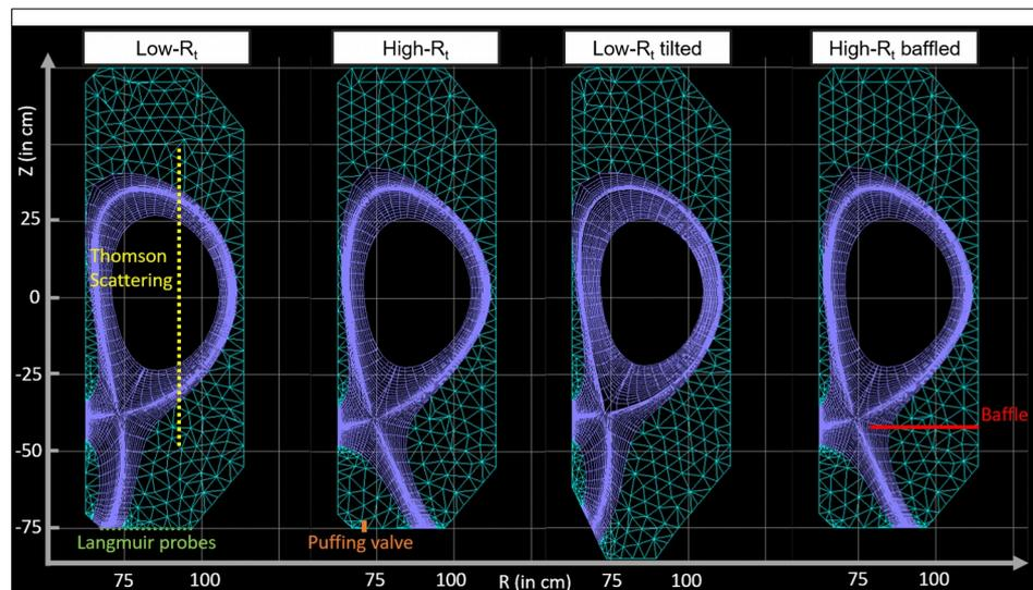
Figure 1: B2.5 plasma grids ("low- $R_t$ ", "high- $R_t$ ", "low- $R_t$  tilted", "high- $R_t$  baffled"). Also shown is the position of the Thomson Scattering measurement, the Langmuir probes which cover the outer target and the position of the gas valve from which we puff particles in the simulation.
