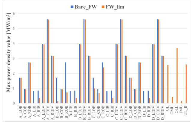
Fig. 7. Heat load peaks on both the bare FW and FW equipped with limiters during the SOF phase.
