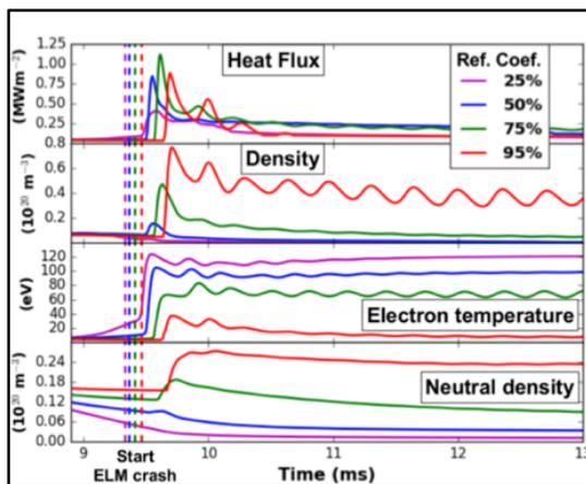
Fig. 3 Evolution of the peak outer target heat flux, density, electron temperature and neutral density for a reflectivity scan.
