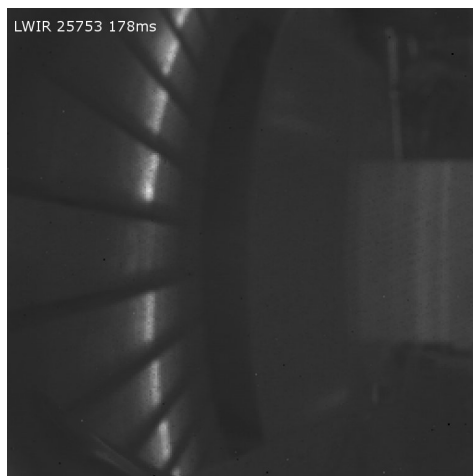
Figure 7: Some of the tiles in the divertor of MAST during shot 25735. The tile in the centre of the image had just been replaced, and the strike point is very faint on this tile compared to the others. This indicates that the new tile had lower emissivity than those which had been exposed to several campaigns already.
