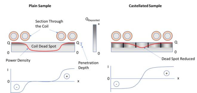
Figure 1 - Illustration of the End/Edge Effects & Coil ‘Dead-Spot’
