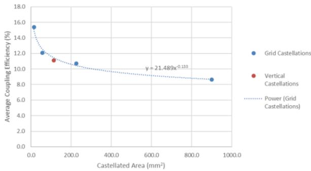
**Figure 6 – Av. Coupling Efficiency Against Castellation Area**
