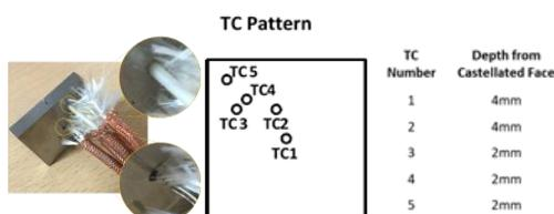
Figure 3 - Thermocouple Installation
