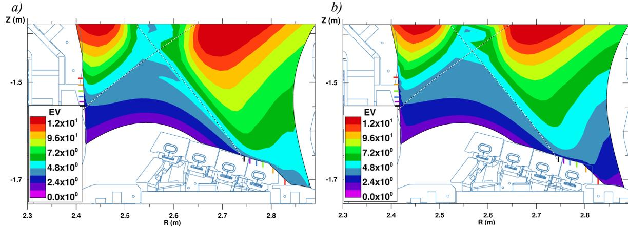
Figure 1. Electron temperatures from simulations with maximum impurity content that use a) ADAS, b) CHEM He II atomic data. Coloured marker lines indicate beginning of field lines used in figures 3 and 5.
