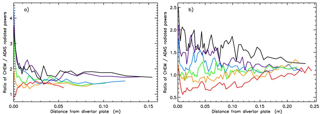
Figure 5. Ratio of the CHEM to ADAS simulated radiated powers along field lines for a) the inner divertor and b) the outer divertor. The coloured marker lines in figure 2 show the starting point of the field lines at the divertor plates.
