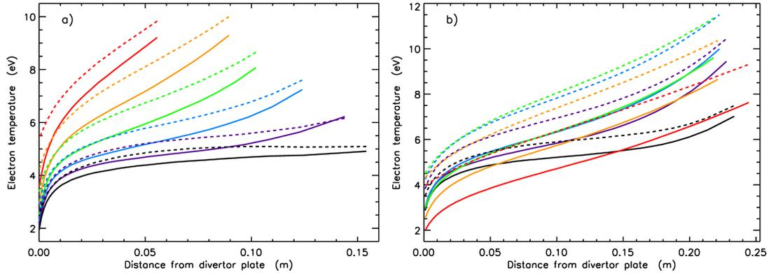
Figure 3. Simulated electron temperatures along field lines for a) the inner divertor and b) the outer divertor: full lines CHEM database, dotted lines ADAS database. The coloured marker lines in figures 1 and 2 show the starting point of the field lines at the divertor plates.
