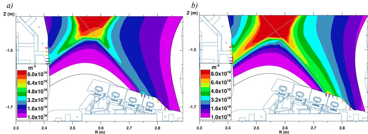
Figure 2. Electron densities from simulations with maximum impurity content that use a) ADAS, b) CHEM He II atomic data. Coloured marker lines indicate beginning of field lines used in figure 3 and 5.
