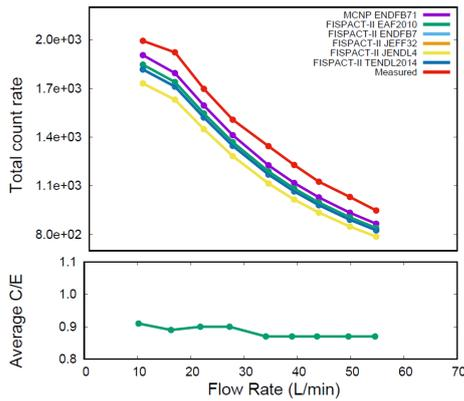
Figure 7: The total count rate calculated for N-16 in the CsI detector with the mock-up at 5 cm for circuit #1 at various water flow rates.
