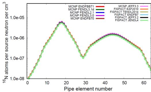
Figure 5: Reaction rates per element for N-16 derived inside the mock-up component, at 2 cm from the FNG source, using MCNP6.1 and FISPACT-II.
