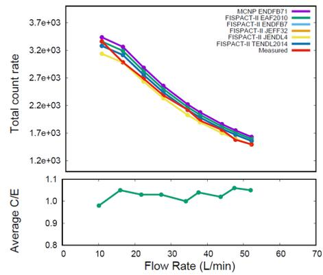
Figure 8: The total count rate calculated for N-16 in the CsI detector with the mock-up at 2 cm for circuit #1 at various water flow rates.
