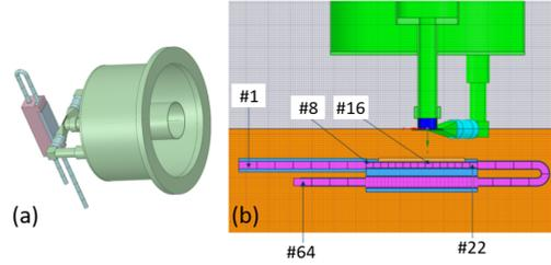
Figure 3: (a) shows a 3D model of the FNG (in green) and the FW mock-up (in purple and blue), (b) a CAD image showing the subdivision of the water regions inside the mock-up with some of the water element numbers indicated.
