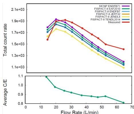
Figure 10: The total count rate calculated for N-16 in the CsI detector with the mock-up at 2 cm for circuit #2 at various water flow rates.
