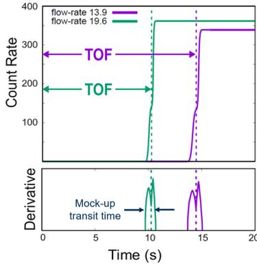
Figure 2: A plot to indicate the methodology used to calculate the TOF. The green and purple curves in the top plot show the activity build-up in the CsI tank for water flow rates 13.9 litres/min and 19.6 litres/min respectively for the ENDFB7.0 nuclear data library, with the mock-up positioned at 2 cm. The bottom plot shows the first derivative of the top plot, and the central dip indicates the TOF between the mock-up and the CsI tank.
