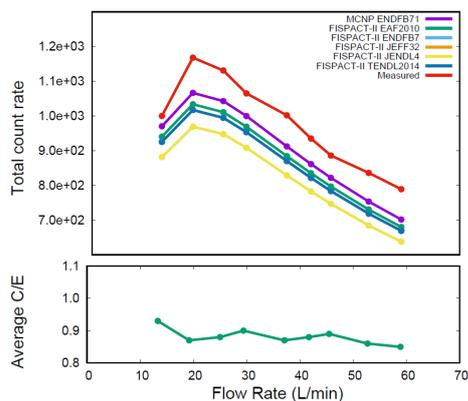
Figure 9: The total count rate calculated for N-16 in the CsI detector with the mock-up at 5 cm for circuit #2 at various water flow rates.
