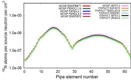
Figure 4: Reaction rates per element for N-16 derived inside the mock-up component, at 5 cm from the FNG source, using MCNP6.1 and FISPACT-II.
