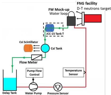
Figure 1: Schematic drawing of the N-16 experimental flowing water circuit at the FNG, circuit #1 (excluding dashed box) consists of the mock-up connected to the CsI tank and the delay tank, whereas circuit #2 also includes the JCC-15 tank in the dashed box.
