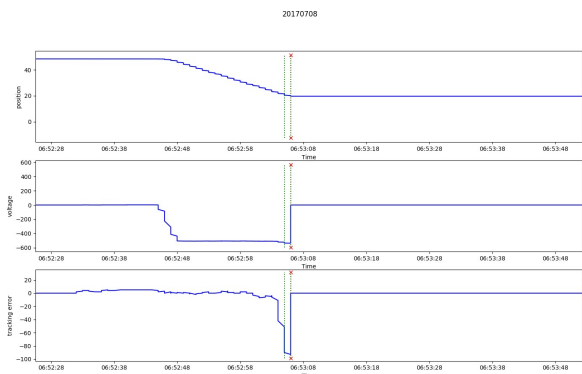
Fig. 10. Joint position, joint motor applied voltage and joint position error as function of time. Gross errors identified by DPGMM are represented with green vertical line. Gross errors identified by the control system are represented with red crosses.
