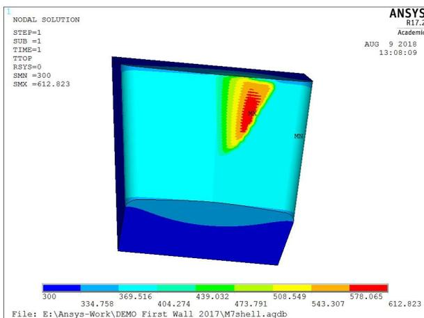
Figure 4: ANSYS result: Temperature distribution [°C] on module 7 surface (nominal case).
