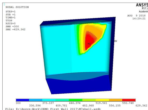
Figure 6: ANSYS result: Temperature distribution [°C] on module 7 surface (nominal case).
