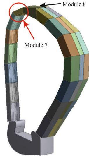
Figure.1. Module 7 location on the inboard blanket segment.
