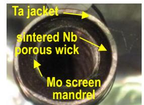
Figure 1. Li-Ta HP before end cap weld.
