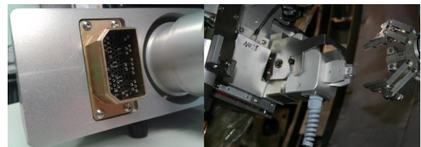
FIG. 1. The ICLS RH chest connector assembly in close-up (showing the high pin-density) and installed in the mating connector on the MASCOT chest (the gripper jaws are visible on the far right).
