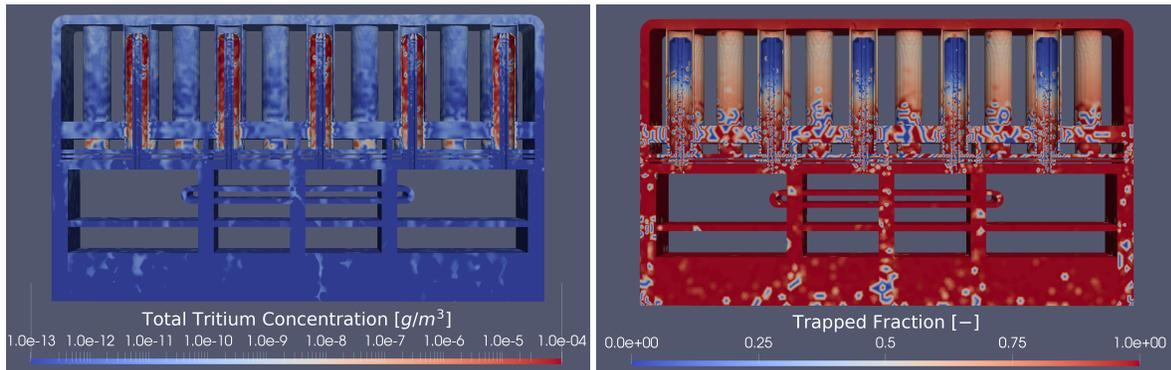
(a) Tritium concentration in steel structure after 1000s of neutron irradiation.
