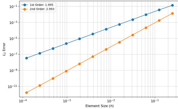
(a) Achlys spatial convergence test for first and second order elements using the method of manufactured solutions.
