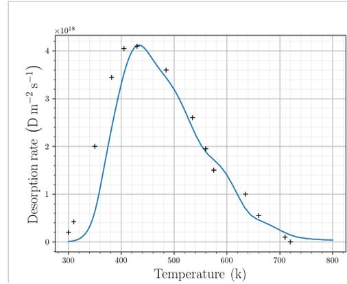
(b) Plot showing a comparison of Achlys against data [26] for desorption rates as a function of temperature.
