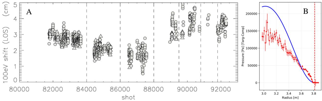
Figure 1: **A.)** Discrepancy between the computed LCFS location with the intershot equilibrium and the measured pedestal foot (100eV location) on the HRTS line-of-sight across several JET campaigns. **B.)** Example of a computed pressure profile (blue) compared to “measured” pressure (red) in a standard magnetics only equilibrium, and a ~3cm gap between the separatrix (dashed) and the pressure pedestal foot.
