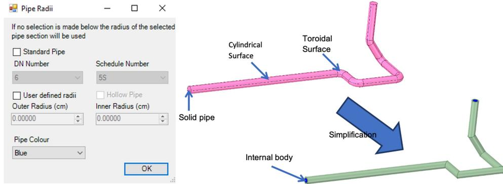
Fig. 4. User interface for the pipe simplification tool (left) together with an example of the original and simplified pipe geometry (right)
