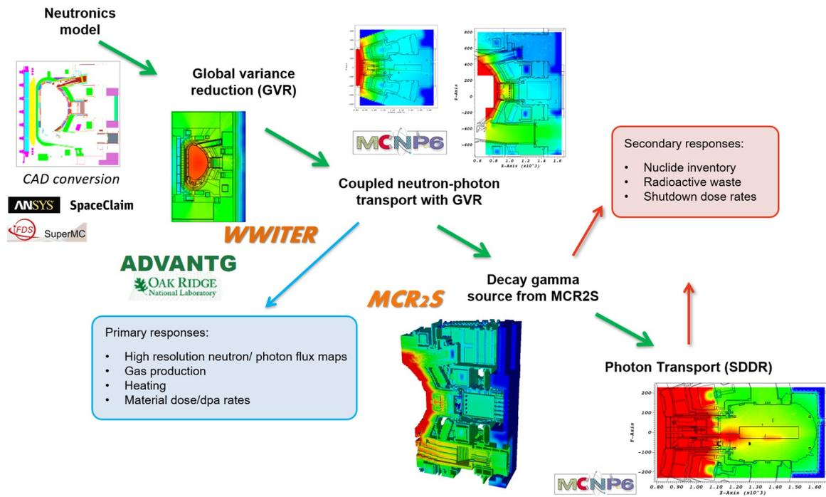
Fig. 2. Schematic overview of the conventional workflow including computational tools used for radiation transport analysis at UKAEA
