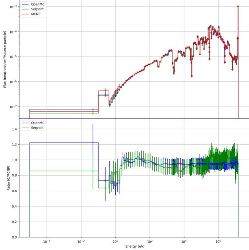
Fig. 8. Comparison of the MCNP, Serpent and OpenMC calculated neutron spectra in the closure plate of the ITER computational port plug. Each code uses an independent method of variance reduction.
