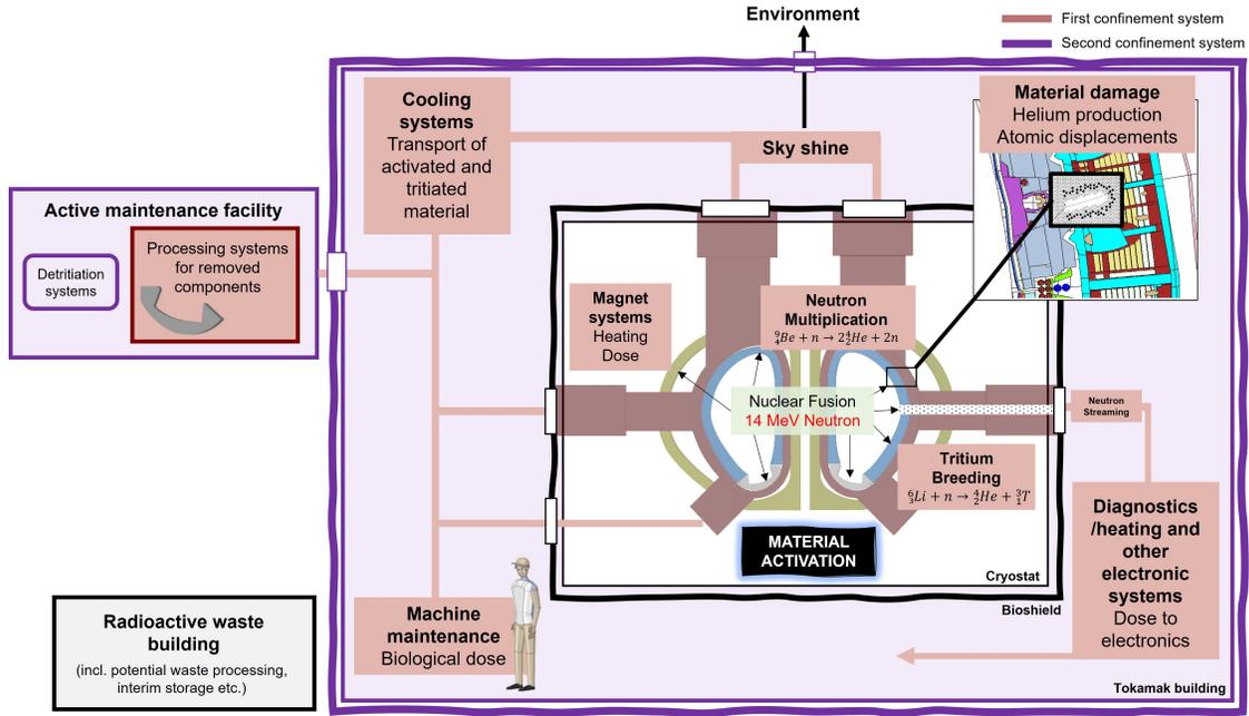
Fig. 1. A schematic illustration of the complex nuclear environment in an operating fusion tokamak. The diagram describes only some of the many complex phenomena that arise from the fusion reaction
