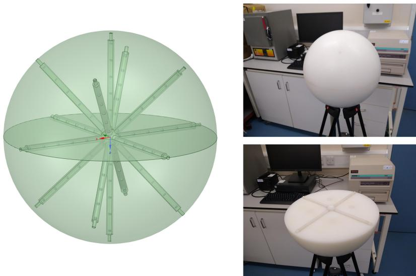
Fig. 10. CAD model (left) and manufactured model of PNS detector (right), with a 30 cm radius sphere of HDPE, 14 arms each with 6 pairs of TLD-600 and TLD-700 badges equally spaced along each arm. On the right hand side, the TLD reader can be seen in the background.
