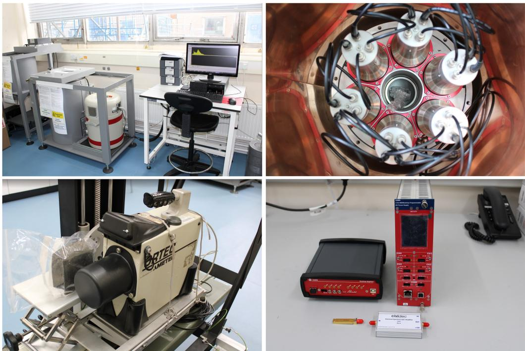
Fig. 9. The broad energy germanium (BEGe) and data acquisition setup in the current on site lab (top left), close up view of the associated Compton suppression system with several sodium iodide detectors (top right), portable Trans-SPEC HPGe (bottom left) and diamond detector with data acquisition system (bottom right)
