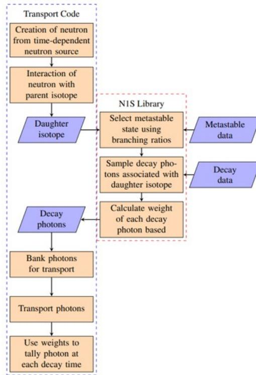
Fig. 5. Flowchart describing the workflow implemented for the Novel-1-Step (N1S) method for determining shut down dose rates
