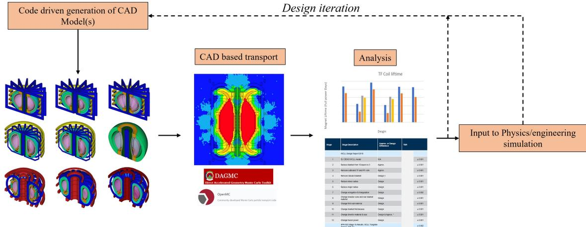
Fig. 6. Schematic overview of the workflow for nuclear analysis based on parameter driven CAD models and CAD based particle transport
