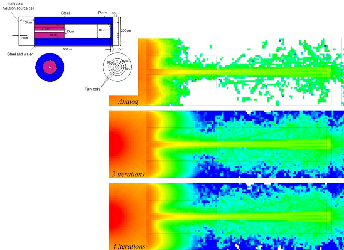
Fig. 7. Neutron flux map for the ITER port plug benchmark in OpenMC using an iterative scheme to generate global weight windows with increasing convergence across the entire mesh. The weight window boundaries are generated with the PS-GVR method.
