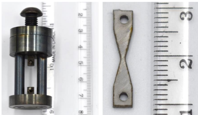
Figure 7: Images of a stress rig and Eurofer-97 waist-section sample (pre-surface preparation)
