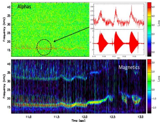
Figure 2. Magnetics and FILD spectrograms show that  $\alpha$ -particle losses correlated with fishbones.
