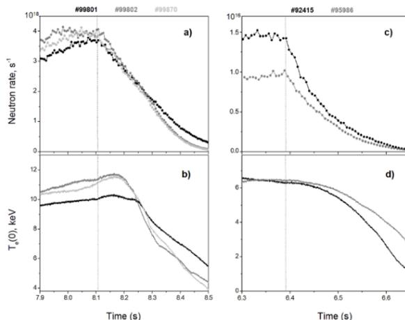
**Figure 1.** (a) and (b) - waveforms of the  $D-T$  JET pulses; (c) and (d) - the deuterium JET pulses (the waveforms were shifted in time to align both NBI afterglow periods). The panels show waveforms of central electron temperatures,  $T_e(0)$ , and measured neutron rates, where the dash line is marking the start of the NBI afterglow period.
