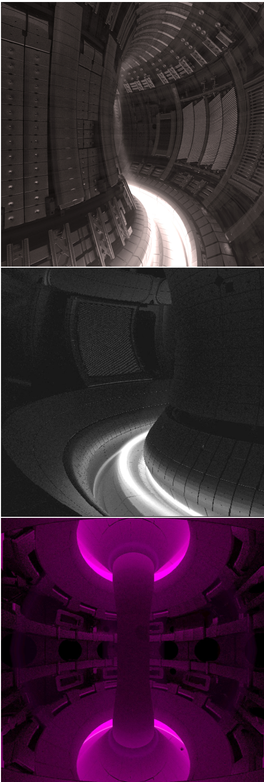
FIG. 8. Simulated images of a) D_{\alpha} emission from JET (black and white), b) D_{\alpha} emission from AUG, and c) predicted visible emission from the Balmer series in MAST-U as would be measured by the mid-plane camera.
